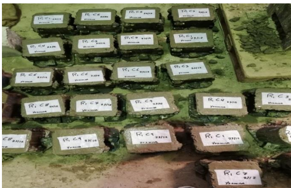
Figure 18: Specimens before and after immersion in MgSO_4
