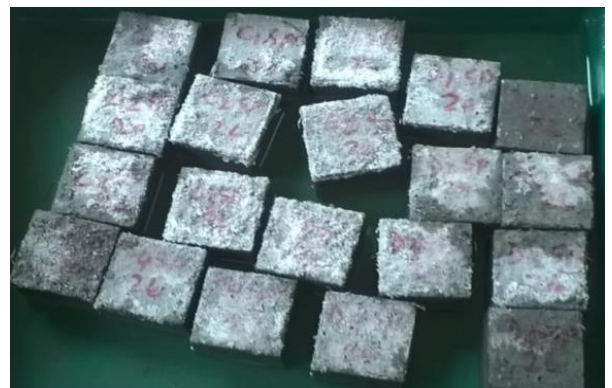
Figure 18: Specimens before and after immersion in MgSO_4
