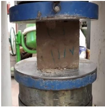
a) Compressive strength test
