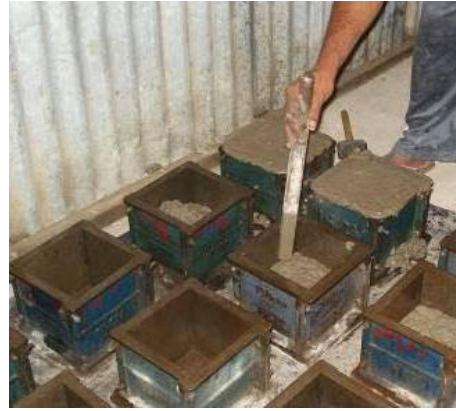
b) compaction of fresh geopolymer concrete
