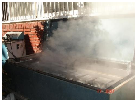
Figure (2), The steam curing tank
