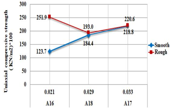
**Fig.21. Analysis of vertical 2 planes rock bridge (Lr) = 2.5**
