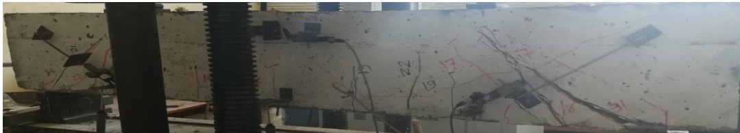
b) Beam content 100%RAC and 10%fly ash at depth ratio 1.1(A-1)
