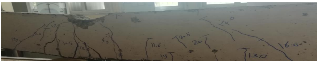
c) Beam content 100%RAC and 1%steel fiber at depth ratio 1.6(B-2)
