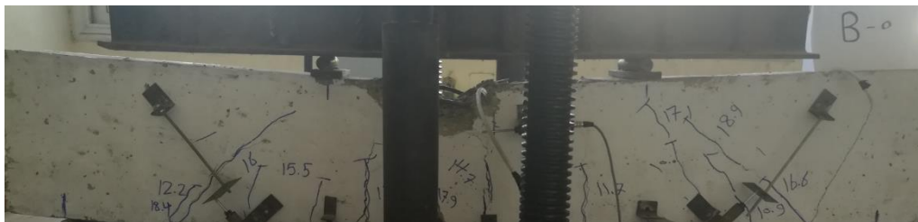
a) Beam content normal concrete at span to depth ratio 1.6(B-0)
