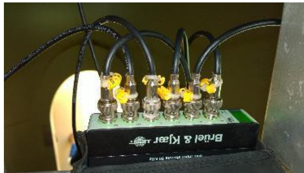
Figure 4: Test equipment (a) LAN-XI unit attached to the ladder
