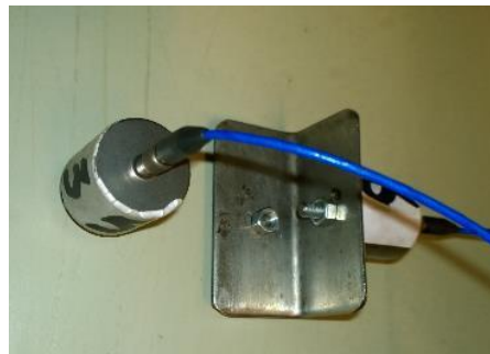
Figure 4: Test equipment (b) PCB accelerometers with magnetic mounting attached to the tower wall
