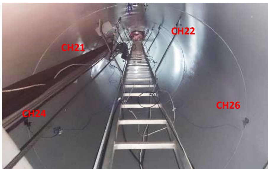
Figure 6: Accelerometers arrangement at level 2 for Vestas N47 Test Setup.
