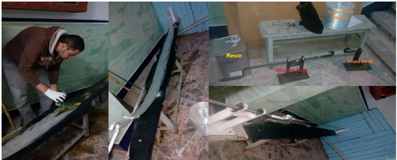
Fig. (2) Stages of locally manufacturing of GFRP bars.
