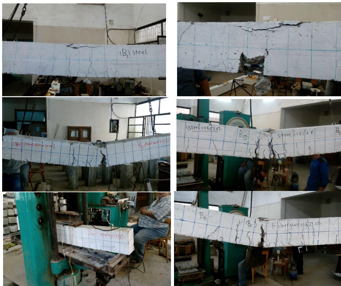
Fig. (8) Crack patterns And Modes of Failure
