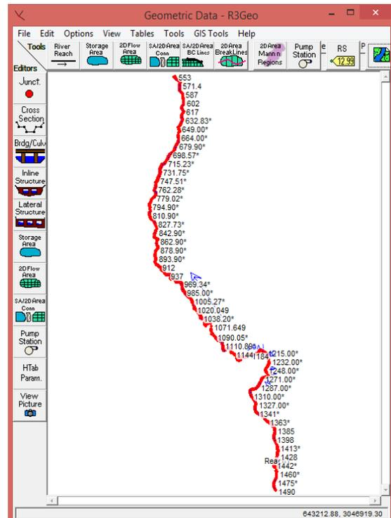
Figure 24: River schematic for four reaches of Nile River in HEC RAS
