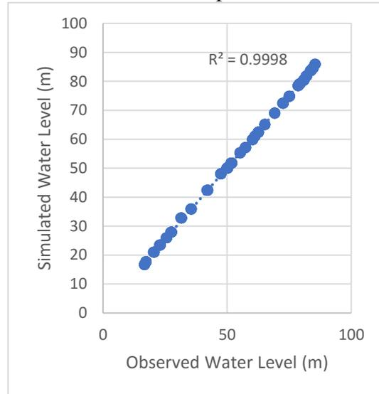
Figure 41: Unsteady Simulation Comparison
