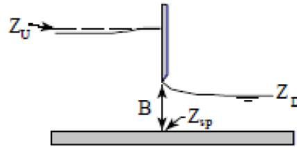
Where  $C$  is the sluice gate discharge coefficient,  $C_{sub}$  is the submerged orifice discharge coefficient,  $W$  is the crest length and  $B$  is the gate opening.
