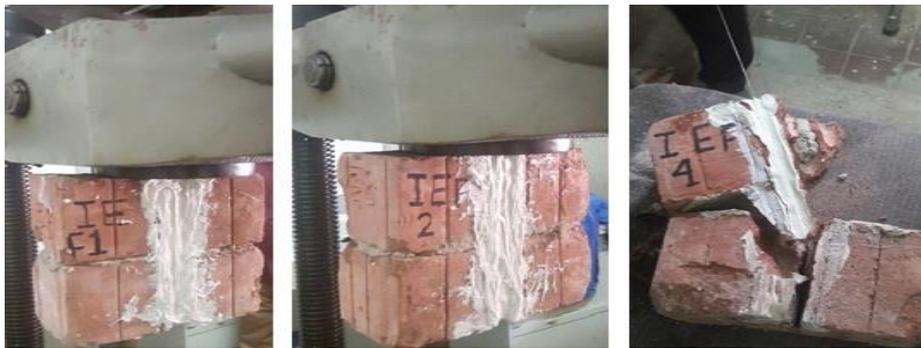
Fig.10. mode of failure of specimens with CFRP NSM
