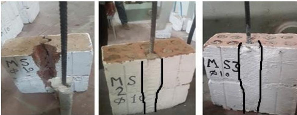
Fig.3. mode of failure of specimens with steel bar 10mm embedded in mortar
