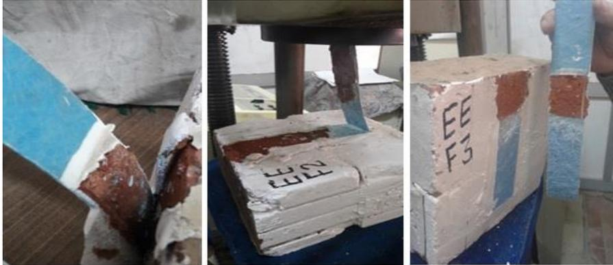
Fig.7. mode of failure of specimens with GFRP bonded externally
