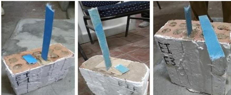
Fig.8. mode of failure of specimens with GFRP NSM
