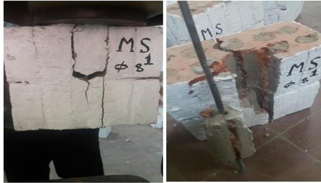
Fig.4. mode of failure of specimens with steel bar 8mm embedded in mortar
