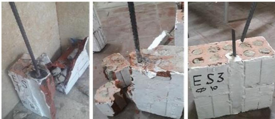
Fig.5. mode of failure of specimens with steel bar 10mm embedded in epoxy
