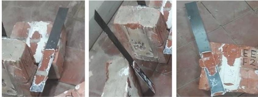
Fig.9. mode of failure of specimens with CFRP bonded externally
