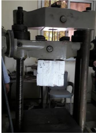
Fig.2. pull-out test set-up
