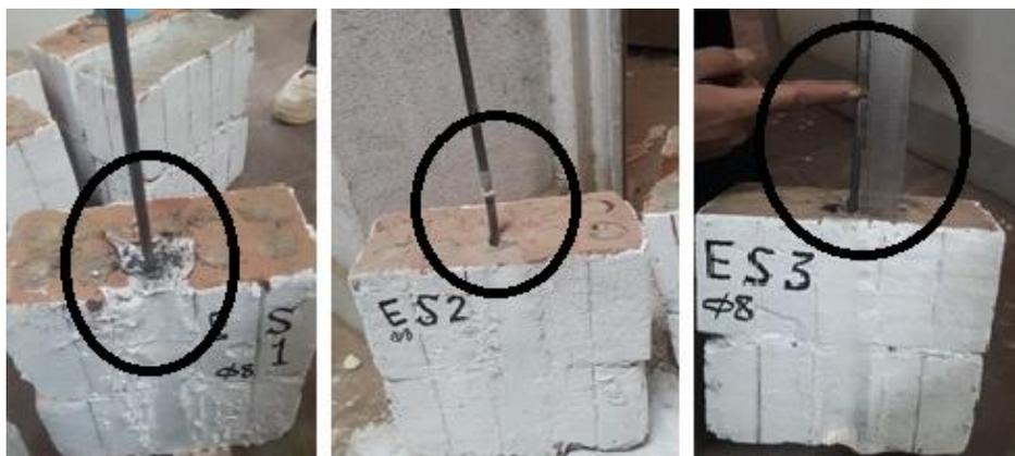
Fig.6. mode of failure of specimens with steel bar 8mm embedded in epoxy
