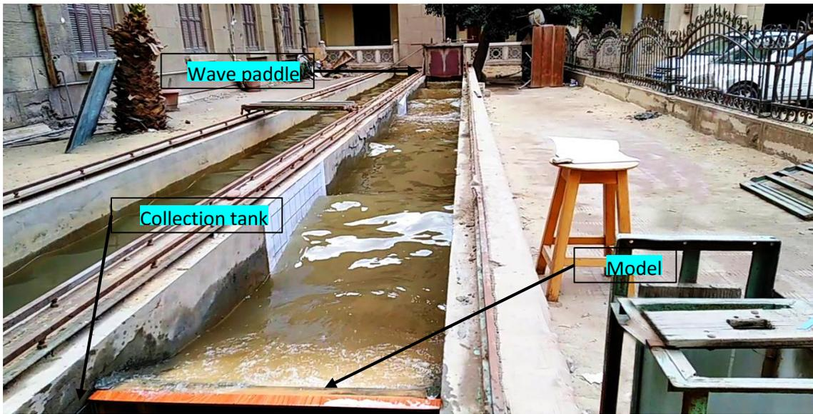
Figure 2 Experimental wave flume
