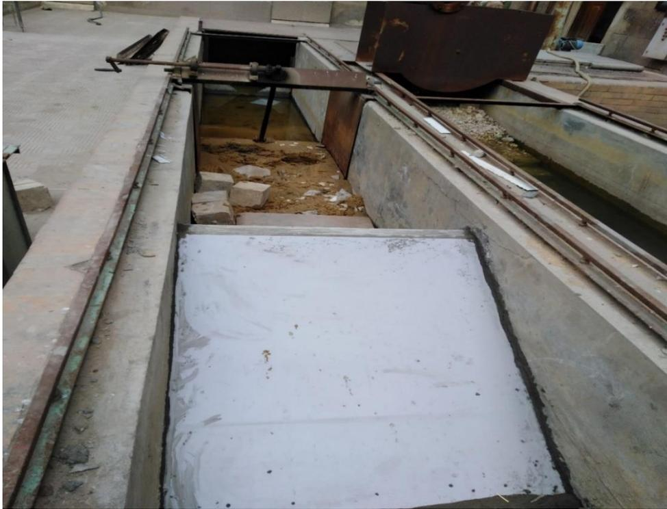
Figure 5 Smooth seawall with front slope 2:1 (H: V).
