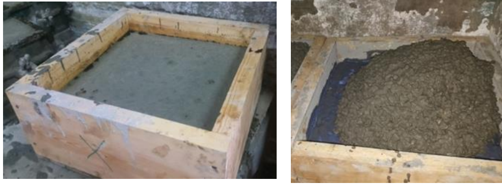
Figure (2) Fabrication of sample substrate concrete and repair concrete
