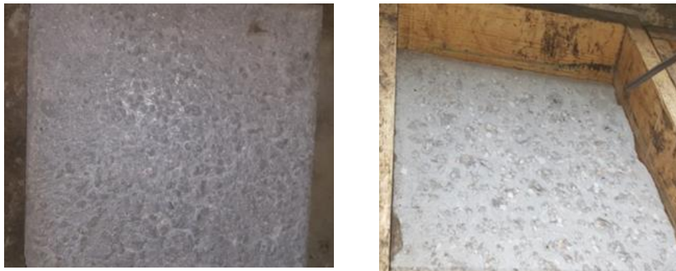
Figure (3) Roughness Surface preparation for substrate concrete
