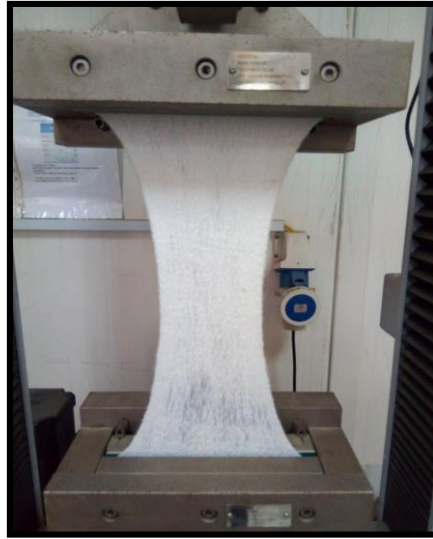
Figure-5: Non-woven geotextile tensile strength test
