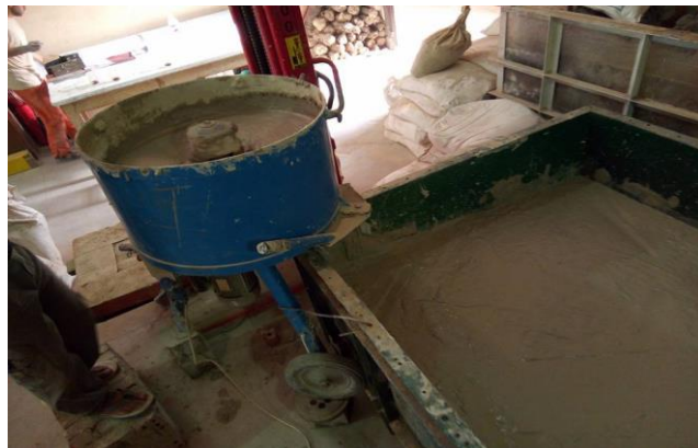
Figure-11: Very soft clay artificially prepared using Kaolinite.
