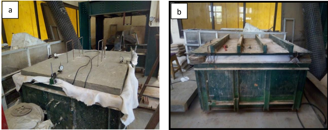
Figure-12: Consolidation process using a) Concrete slab and b) Balloon
