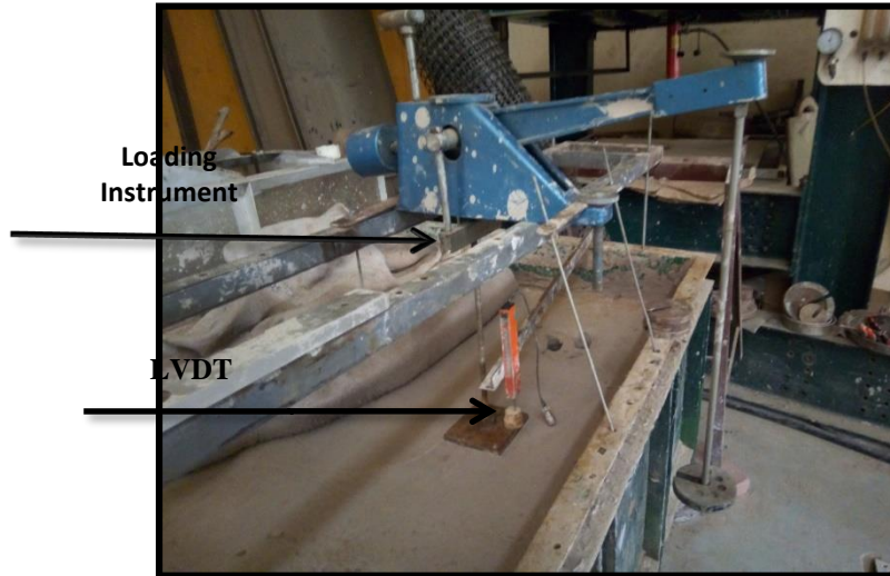
Figure-9: The loading system with measuring instruments for the experimental model.
