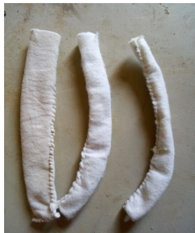
Figure-13: Encasement geotextile after preparation
