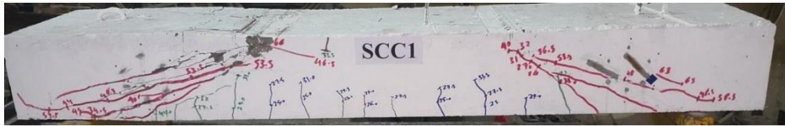
Figure.4a, Crack pattern for Specimen SCC1.
