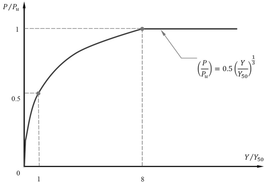
**Figure 1: Soft clay (Matlock) model.**
