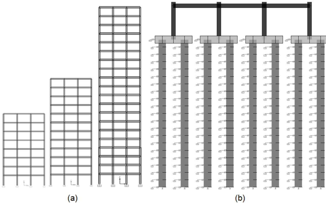
**Figure 2: (a) SAP2000 2D-Model - Without SPSI. (b) SAP2000 2D-Model - With SPSI.**
