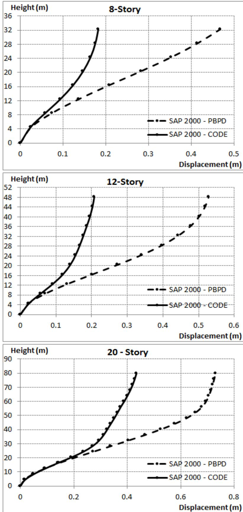
Figure 3: Floor Displacement - Without SPSI - Fixed-base support, for 8, 12 and 20 story.
