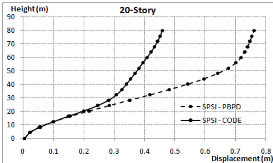
Figure 4: Floor Displacement - With SPSI, for 8, 12 and 20 story.
