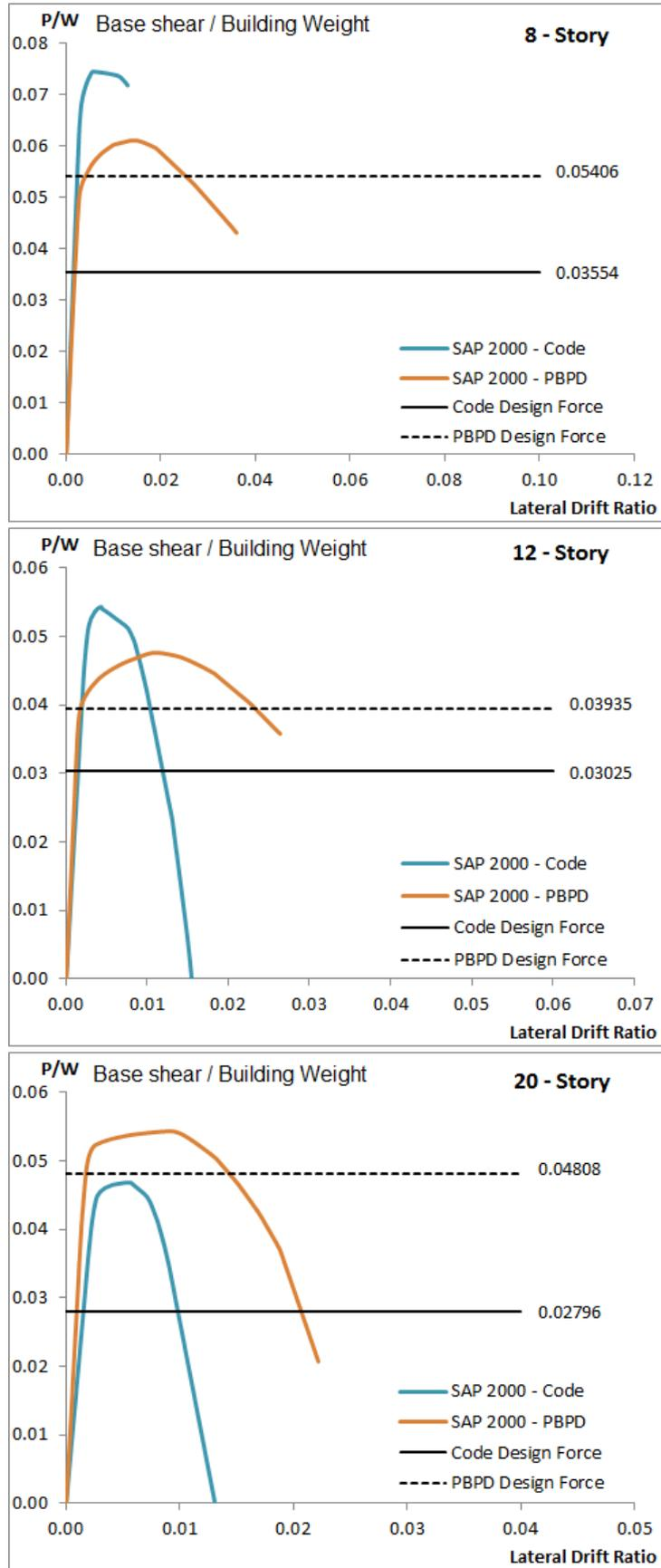
Figure 5: Base shear ratio versus Lateral drift ratio for fixed base, for 8, 12 and 20 story.
