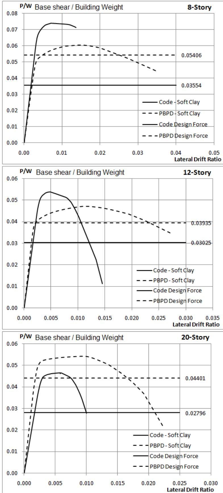
Figure 6: Base shear ratio versus Lateral drift ratio considering SPSI.
