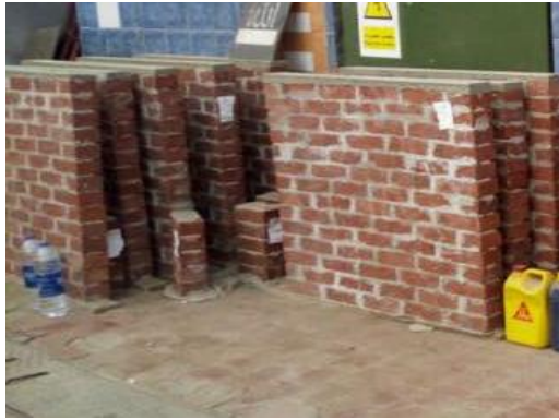
Prisms and Walls before testing
