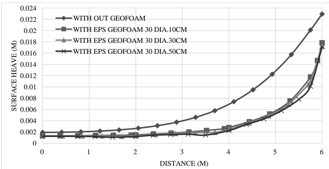
**Fig.12** Surface heave with/without using EPS30 geofoam piles with different diameter after ten days.
