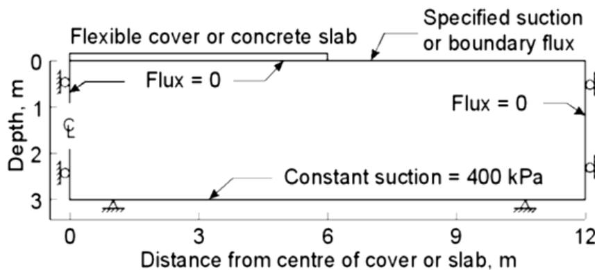
**Fig.1** Case Geometry and the Boundary Conditions for Seepage and Stress-deformation Analysis (Fredlund & Vu, 2003).
