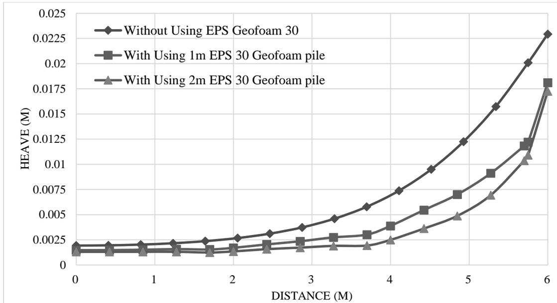
**Fig.12** Surface heave with/without using EPS30 geofoam piles with different length after ten days.
