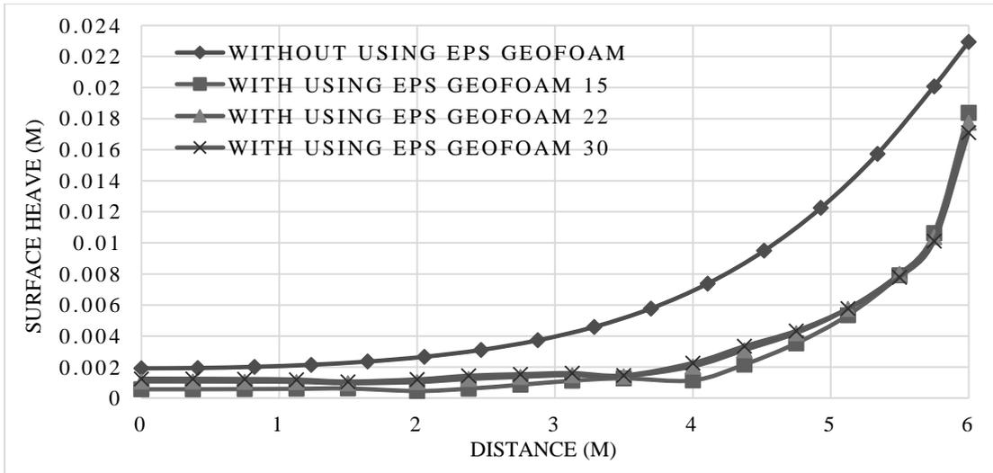
**Fig.11** Surface heave with/without using EPS geofoam piles with dia.50cm with different densities after ten days.
