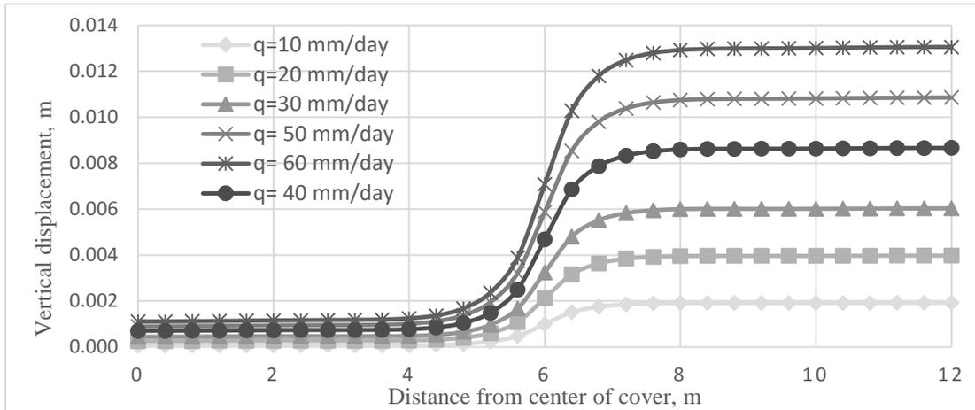
**Fig.5** The Vertical Displacements at the ground surface after one day of infiltration for various infiltration rates using SIGM/W program
