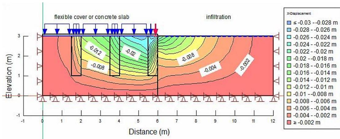
**Fig.9** The Horizontal displacement after ten days using 50 cm EPS15 geofoam piles.
