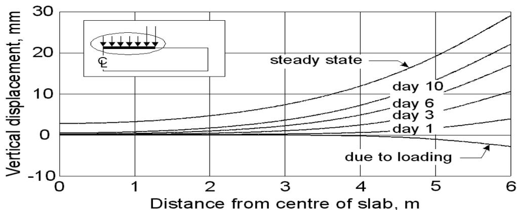
**Fig.4** Vertical displacement of the slab due to infiltration with time (Fredlund & Vu, 2003).
