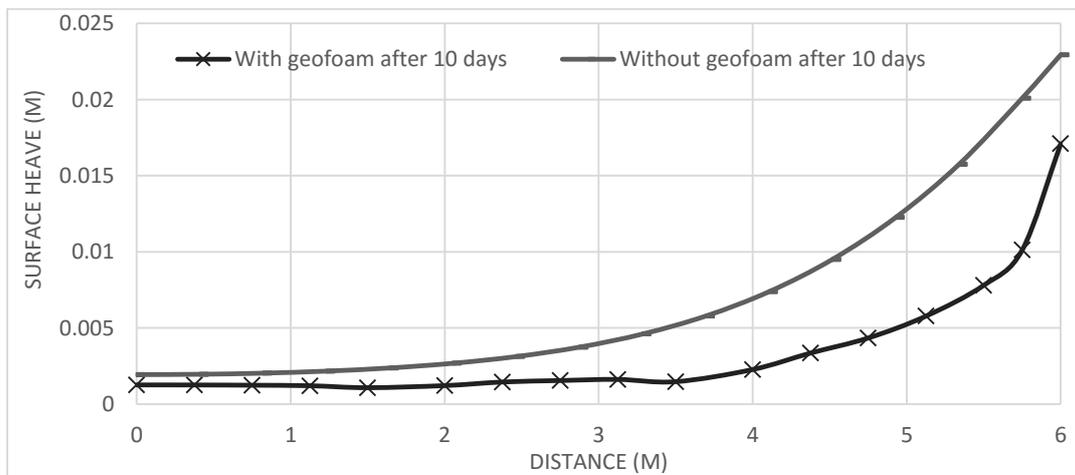
**Fig.10** Surface Heave after ten days with/without using 50 cm diameter EPS 30 geofoam piles.
