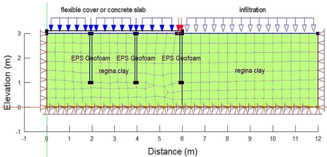
**Fig.7** Simulated Finite element model with EPS geofoam Piles arrangement
