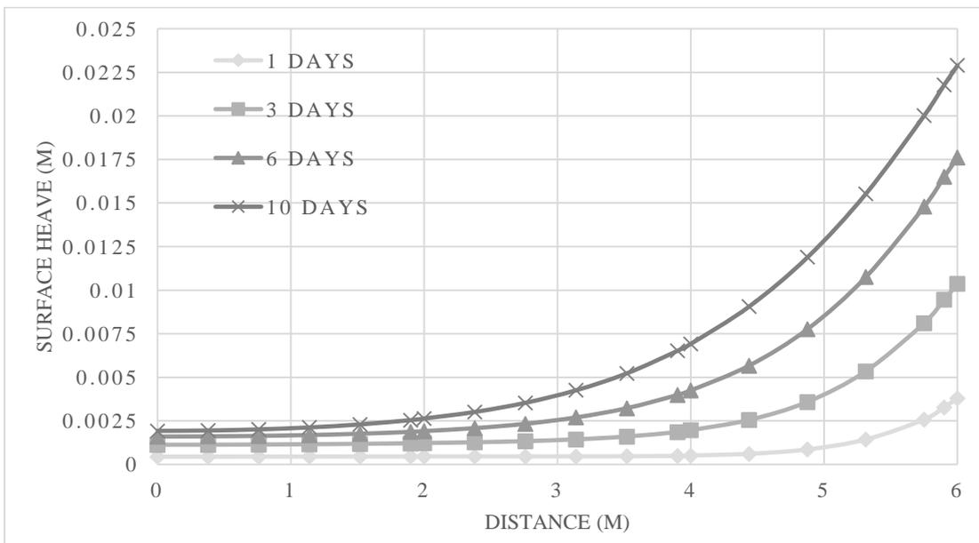
**Fig.6** Vertical movement of the slab due to infiltration with time using SIGMA/W program.
