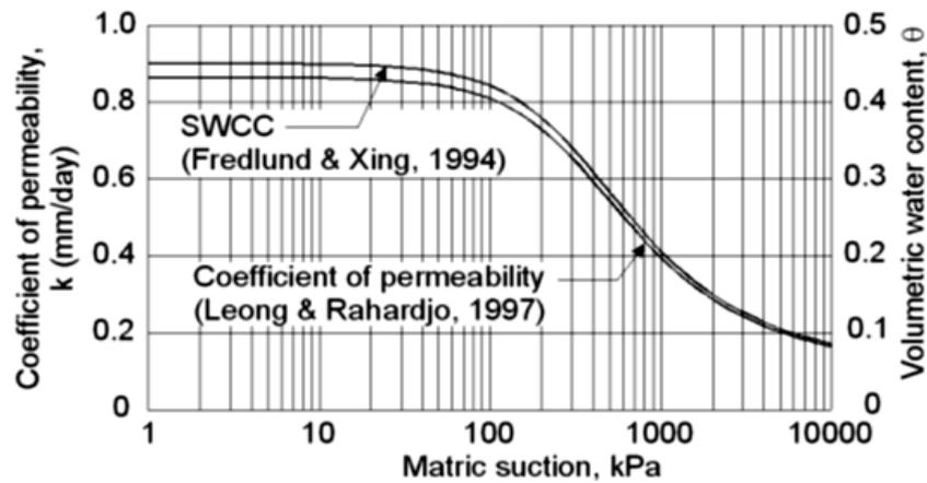
**Fig.2** The Permeability Function and Soil Water Characteristic Curve (SWCC) (Fredlund & Vu, 2003).
