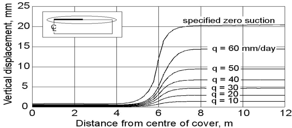
**Fig.3** Vertical displacements of the ground surface after one day of different infiltration rates (Fredlund & Vu, 2003).
