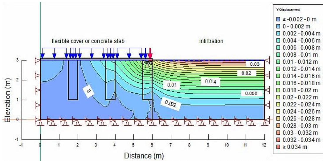
**Fig.8** The Vertical displacement after ten days with using 50 cm EPS15 geofoam piles.
