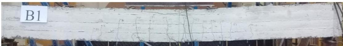
Fig.7: Crack Pattern and Failure for Specimen B1 (NRU-0.70).
