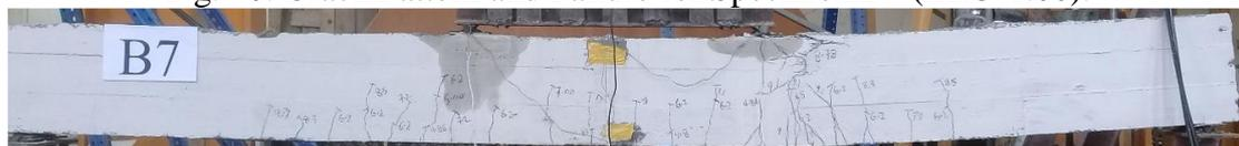
Fig. 11: Crack Pattern and Failure for Specimen B7 (LRU-0.56).
