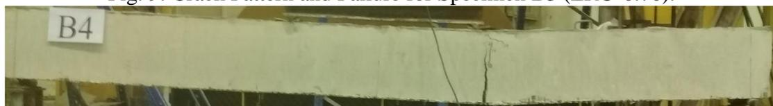
Fig. 10: Crack Pattern and Failure for Specimen B4 (LRU-1.00).
