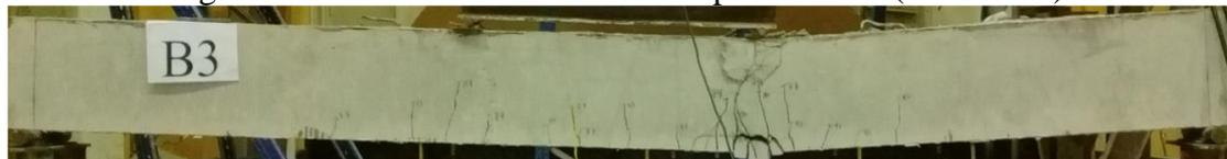
Fig. 9: Crack Pattern and Failure for Specimen B3 (LRU-0.70).
