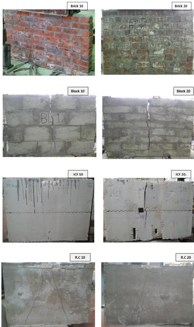
Figure (2) Cracking Pattern and failure mode of the test specimens
