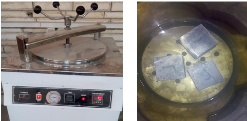
Fig .5.Steam curing using autoclave
