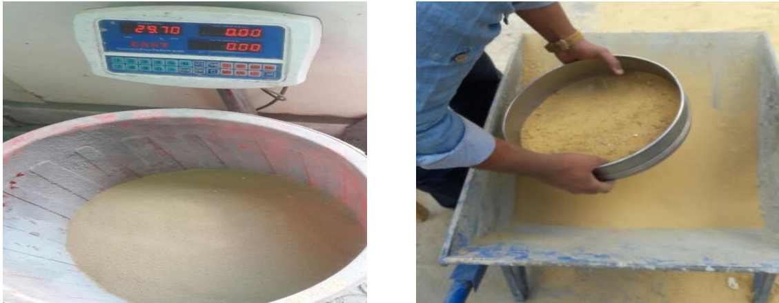
Fig.2.Fine sand passes from sieve (600 \mu m)
