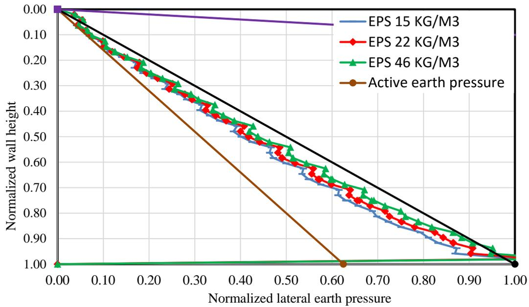
**Figure 10:** Numerical results for 12m basement wall with using EPS geofoam thickness 20 cm with backfill relative density 75%.
