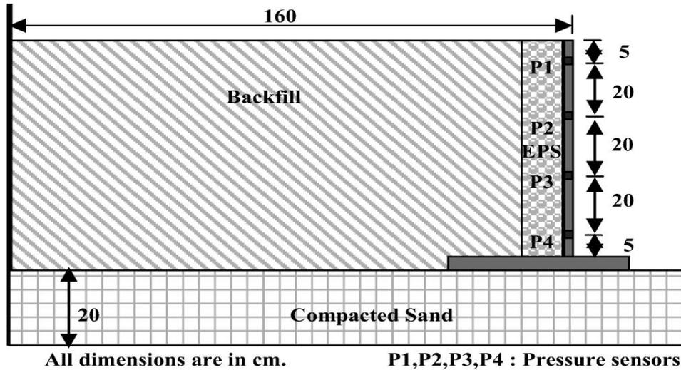
**Figure 1:** Cross section of the test set up. (Ertugrul and Trandafir 2011).
