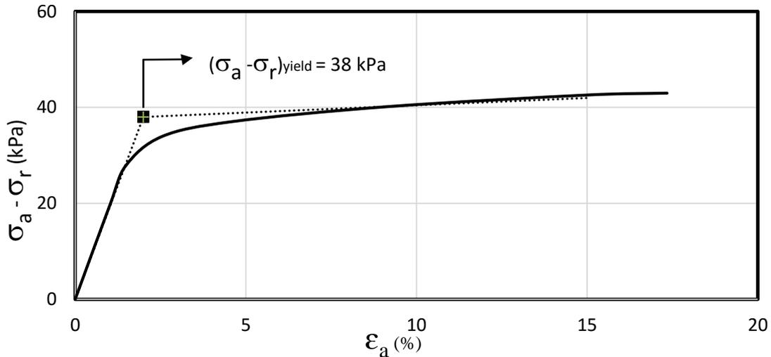
**Figure 2:** Results of uniaxial compression test ( $\sigma_r = 0$ ) on geofoam (Ertugrul and Trandafir 2011)
