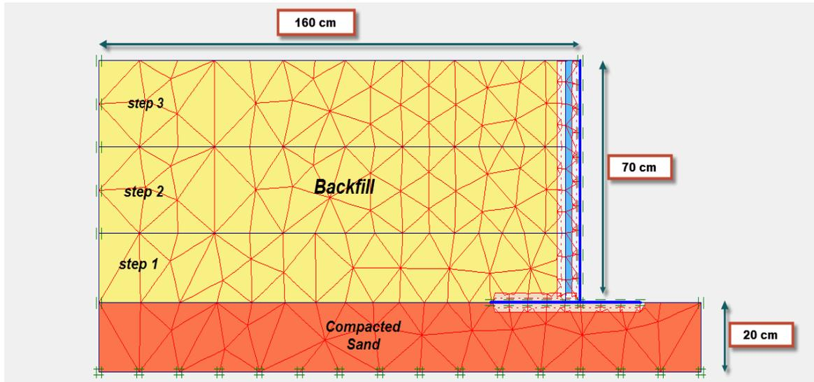
**Figure 5:** Plaxis grid for modeling of retaining wall
