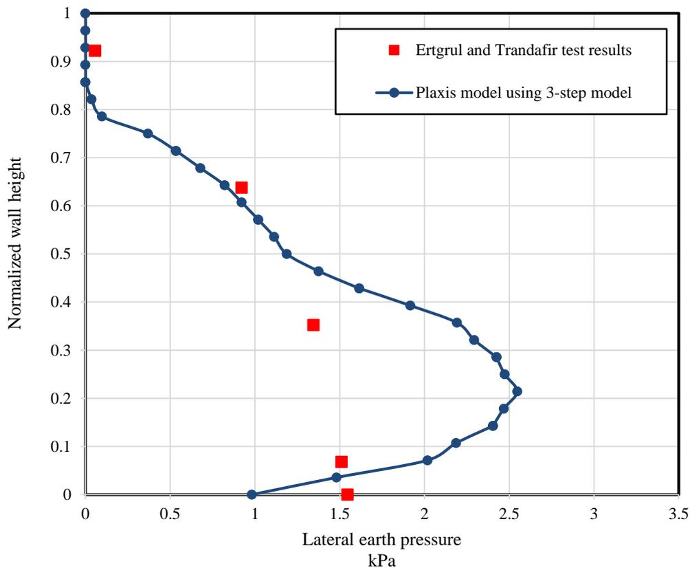
**Figure 8:** Numerical Plaxis model results for 3-steps model with ( $t/h=0.28$ ).
