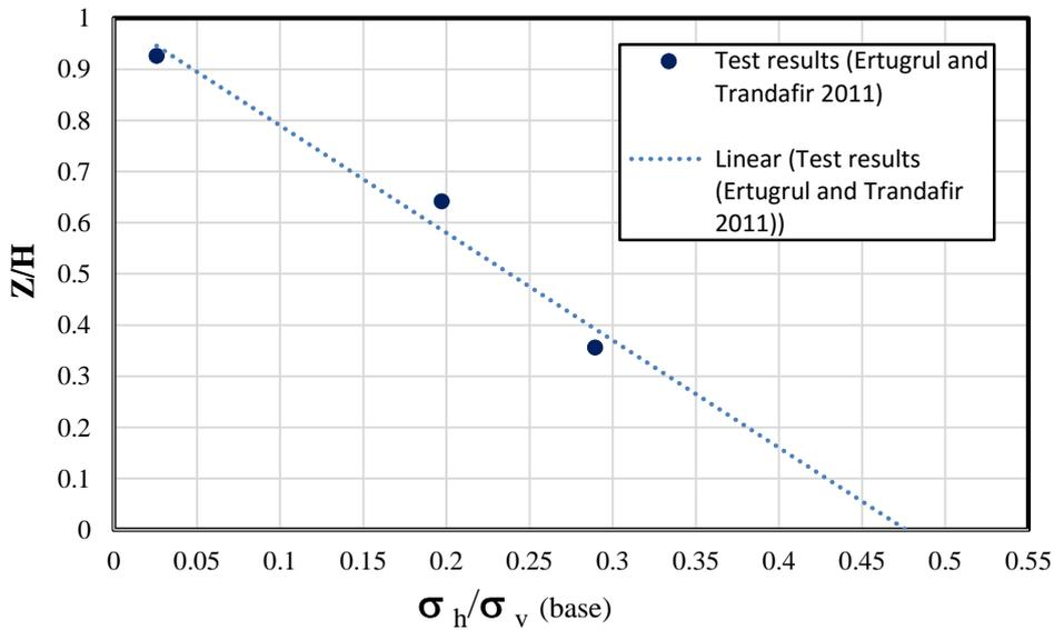
**Figure 4:** Test results for retaining wall without using EPS geofoam after (Ertugrul and Trandafir 2011).
