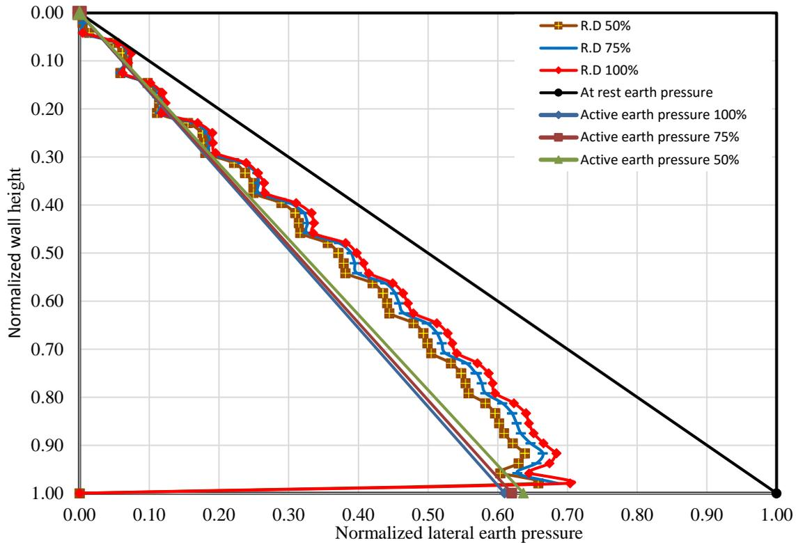
**Figure 15:** Numerical results for 12m basement wall with using EPS geofoam thickness 100 cm with EPS geofoam density  $45.7 \text{ kg/m}^3$  for variable backfill relative density.
