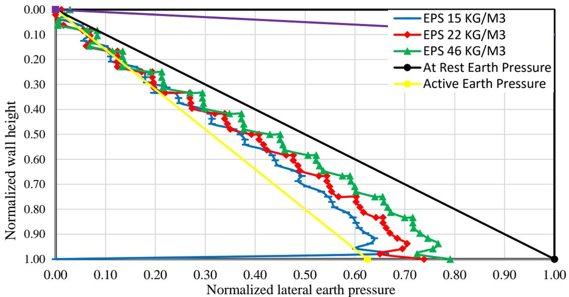
**Figure 11:** Numerical results for 12 m basement wall with using EPS geofoam thickness 100 cm with backfill relative density 75 %
