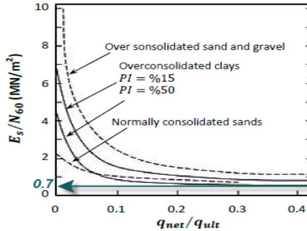
**Figure 3.b:** Relation between  $E_s - \text{SPT-N}$  and  $(q_{\text{net}}/q_{\text{ult}})$  after (Stroud 1989)
