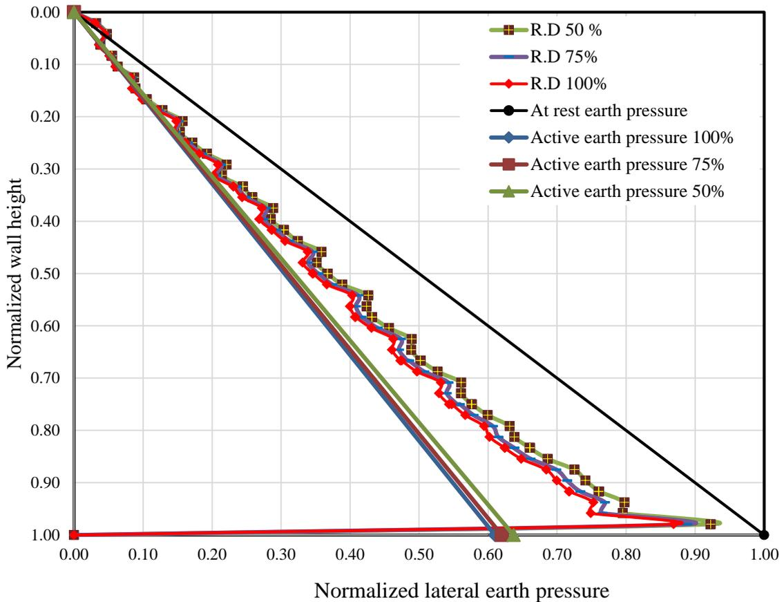
**Figure 14:** Numerical results for 12m basement wall with using EPS geofoam thickness 20 cm with EPS geofoam density  $45.7 \text{ kg/m}^3$  for variable backfill relative density.
