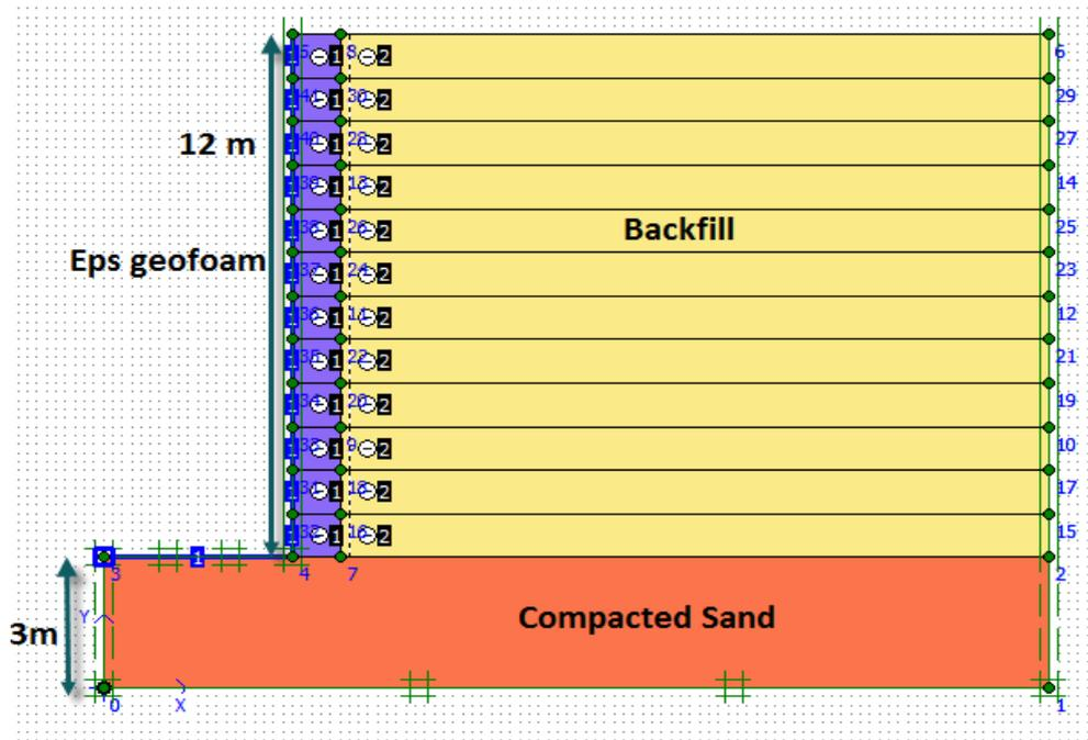
**Figure 9:** Cross-sectional sketch of the Parametric models
