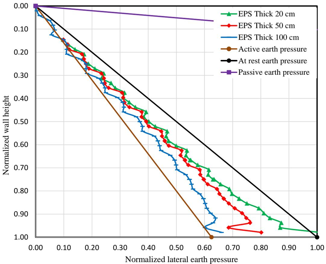
**Figure 12:** Numerical results for 12m basement wall with using EPS geofoam density  $14.4 \text{ kg/m}^3$  with backfill relative density 75 %.
