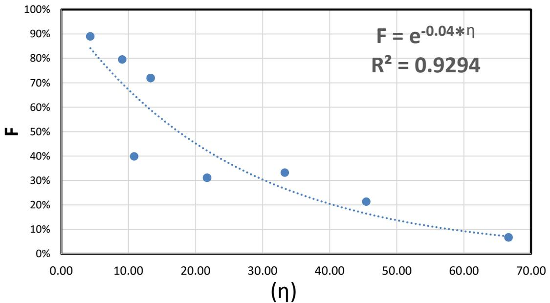
**Figure 14:** The relation between EPS geofoam stiffness factor and normalized lateral earth pressure factor.
