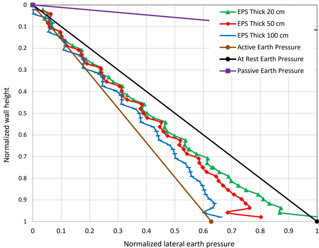
**Figure 13:** Numerical Results for 12m Basement wall with using EPS geofoam Density 45.7 kg/m<sup>3</sup> with Back Fill Relative Density 75 %.
