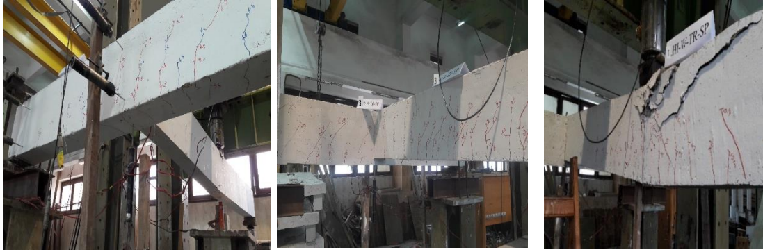
Figs. (4) General Crack Patterns of Tested T-shaped Specimens
