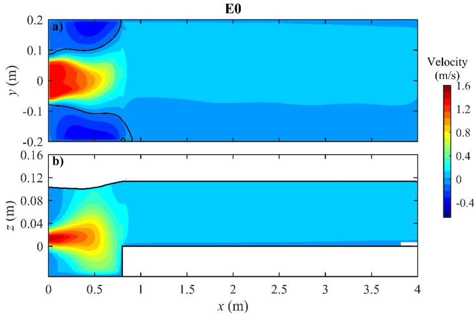
**Figure (2) Distribution of longitudinal velocity over horizontal plane at height  $z = 0.02$  m above bed and a longitudinal profile at  $y = 0$  for run E0. Parameters were  $L = 0.8$  m,  $s = 0.053$  m,  $F_r = 3.0$ ,  $h_e = 0$  and  $b_e = 0$ .**
