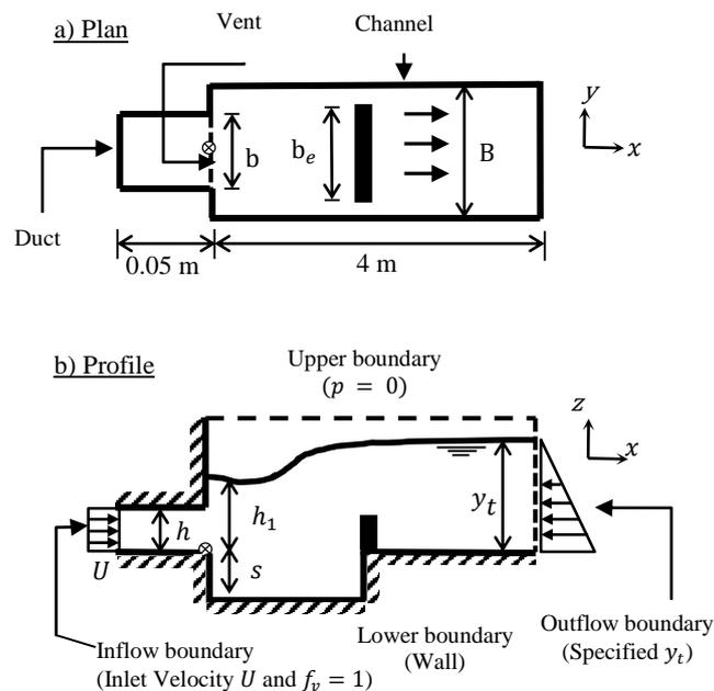
**Figure (1) Schematic of a stilling basin with an end sill downstream of an abrupt expansion. Shown are the geometry and boundary conditions for the numerical domain in a) plan view and b) profile view through vent. Coordinate system  $x$ ,  $y$ , and  $z$  has the origin indicated by the marker  $\otimes$ .**
