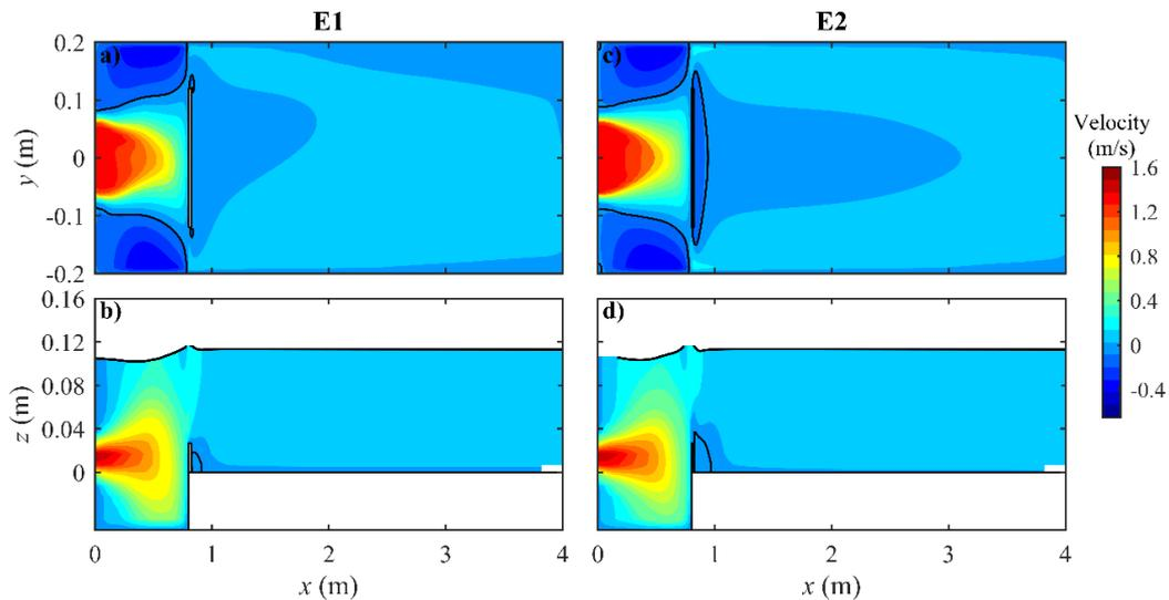
**Figure (3) Distribution of longitudinal velocity over horizontal plane at height  $z = 0.02$  m above bed and a longitudinal profile at  $y = 0$  for run E1, and run E2.**
