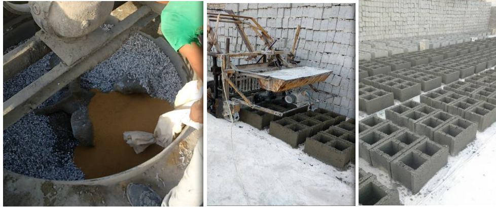
Fig (2) show the production process of hollow concrete blocks
