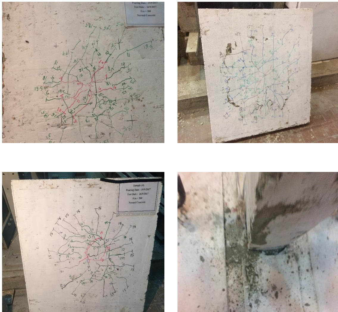
Fig.5 Crack pattern of slab specimens.
