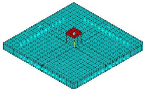
Figure 9 : Loads and Boundary Conditions of Flat Slab Models.
