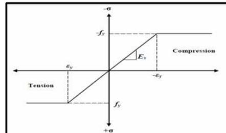
Figure 8 : Stress-Strain Curve for Steel Reinforcement.
