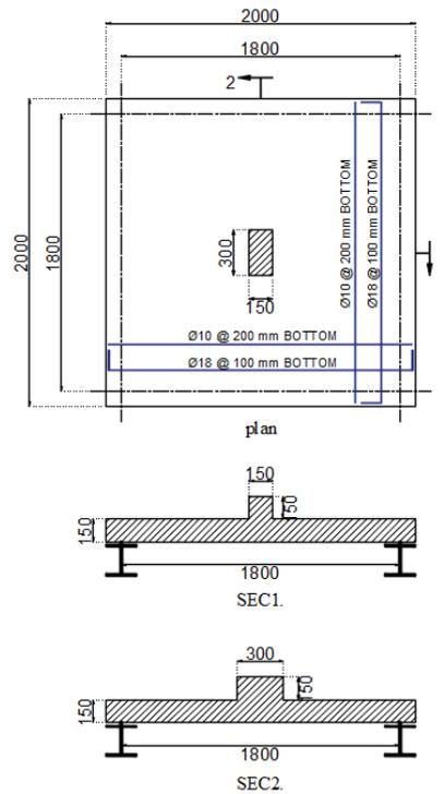
Figure 11 : Specimen with Column Aspect Ratio 2:1 (Dimensions in mm).
