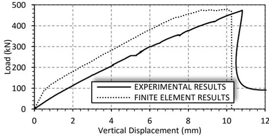
Figure 20 : The Load Displacement Diagram for Exp. and F.E. Results of Specimen (S0).
