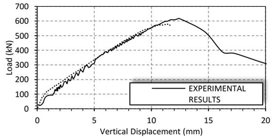
Figure 23 : The Load Displacement Diagram for Exp. and F.E. Results of Specimen (SC3X8-d3).
