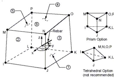
Figure 1 : Solid65– 3-D reinforced concrete solid (ANSYS 12.0).
