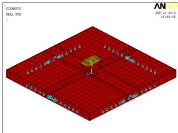
Figure 3 : Modeling of Flat Slab Which Connected with Rectangular Column (2:1).
