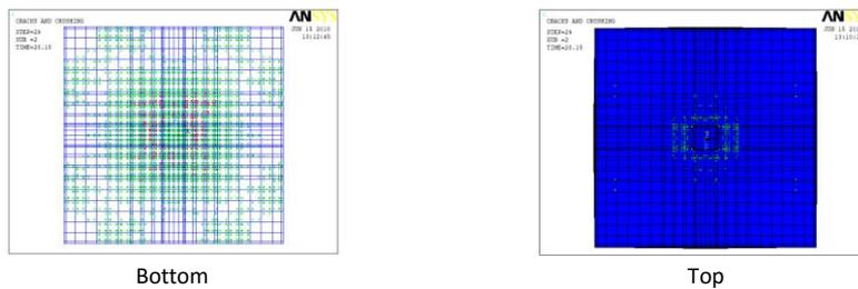
**Figure 14 : The Crack Pattern and Failure Mode at The Bottom and Top of Specimen (SC3X8-d2).**
