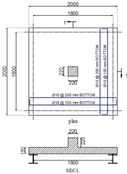
Figure 10 : Specimen with Column Aspect Ratio 1:1 (Dimensions in mm).
