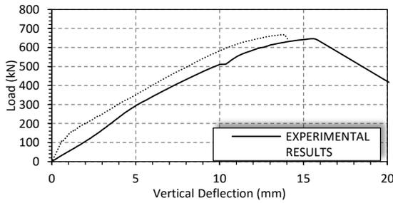
Figure 22 : The Load Displacement Diagram for Exp. and F.E. Results of Specimen (SC3X8-d2).
