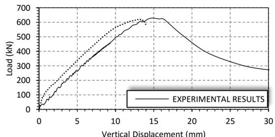
Figure 27 : The Load Displacement Diagram for Exp. and F.E. Results of Specimen (RC3X8-d3).
