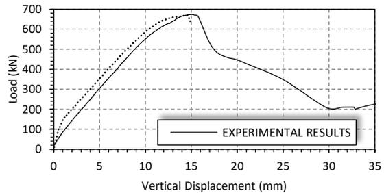
Figure 25 : The Load Displacement Diagram for Exp. and F.E. Results of Specimen (RC3X8-d1).
