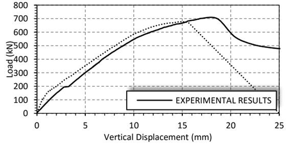
Figure 21 : The Load Displacement Diagram for Exp. and F.E. Results of Specimen (SC3X8-d1).
