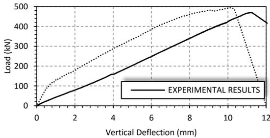
Figure 24 : The Load Displacement Diagram for Exp. and F.E. Results of Specimen (R0).
