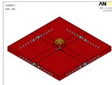
Figure 2 : Modeling of Flat Slab Which Connected with Square Column (1:1).
