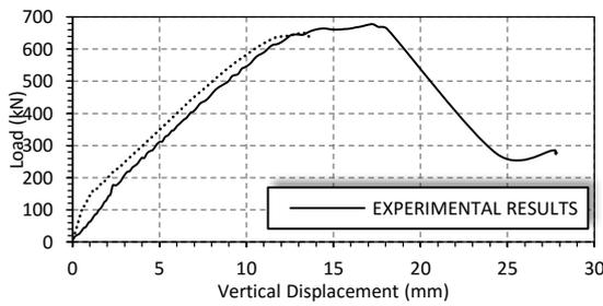
Figure 26 : The Load Displacement Diagram for Exp. and F.E. Results of Specimen (RC3X8-d2).
