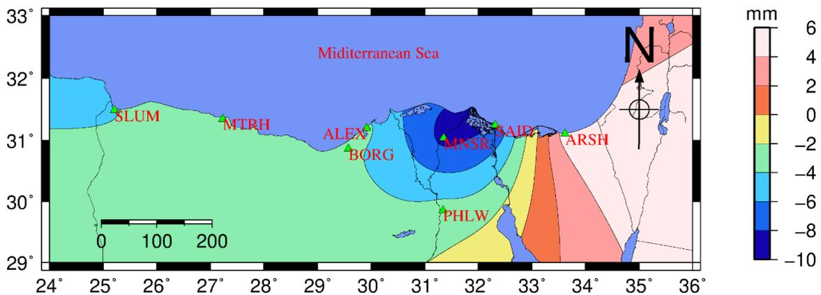
**Fig. 6 The contour map of vertical velocity distribution of the north Egypt network**
