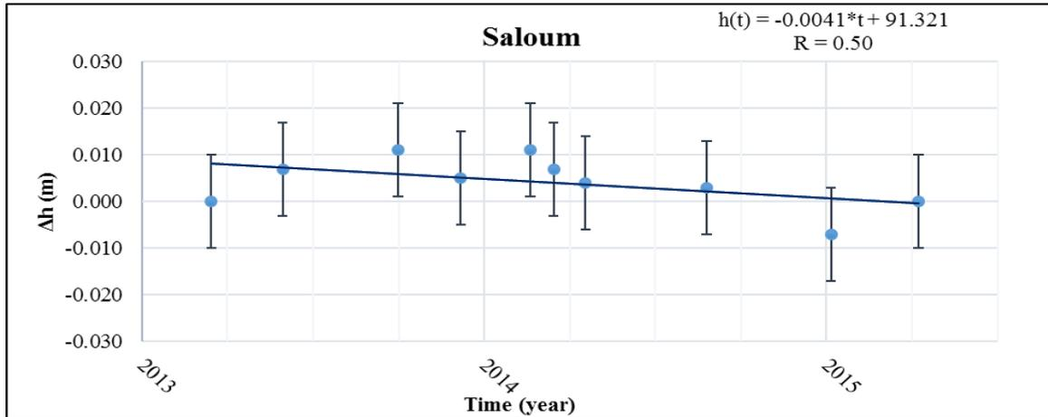
**Fig. (3 – h) Linear Trends of Vertical Movements at SLUM station**
