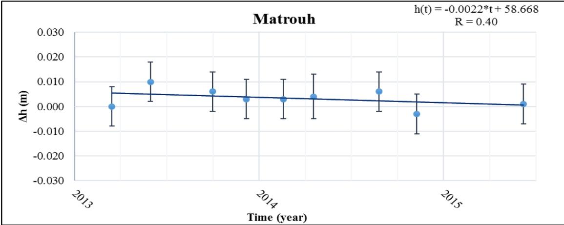
**Fig. (3 – e) Linear Trends of Vertical Movements at MTRH station**
