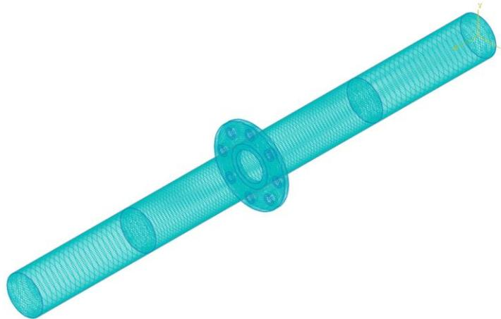
**Figure 7 Finite element model of unstiffened joint**
