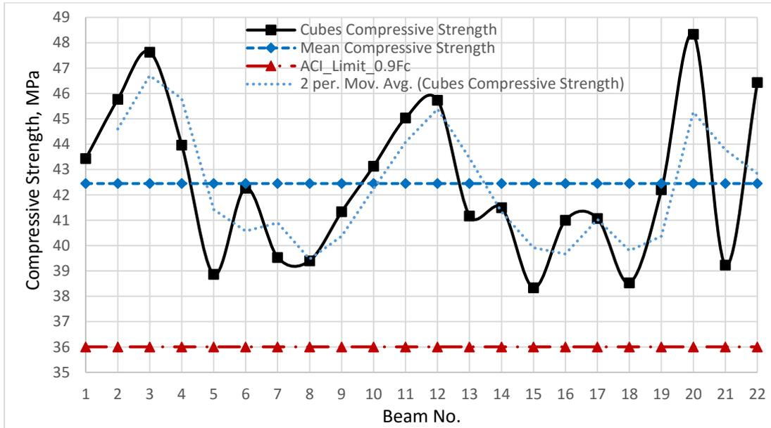
Figure 4: Statistical analysis of individual strength test for 22 beams
