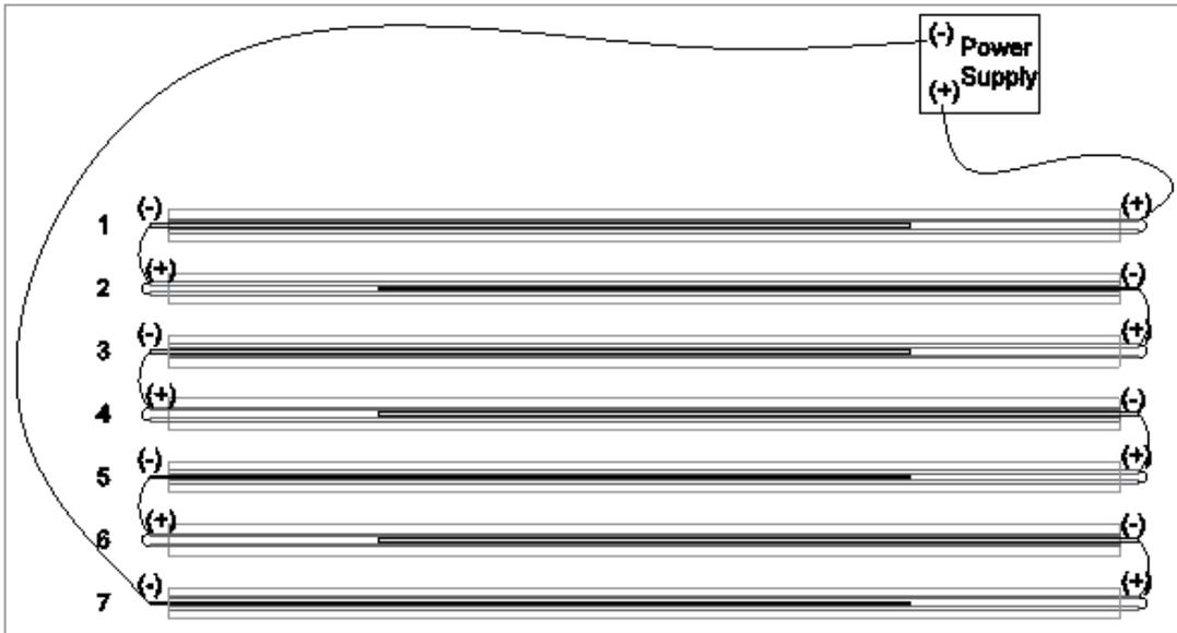
**Figure 2: Schematic drawing for the corrosion circuit set-up**
