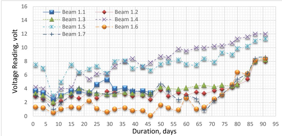
**Figure 7: Voltage readings (Volts) vs. duration (days) for the C-ow beams**
