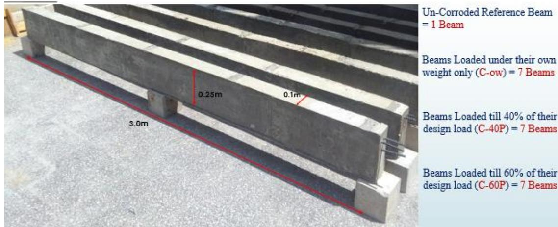
**Figure 1: Typical beam dimensions**
