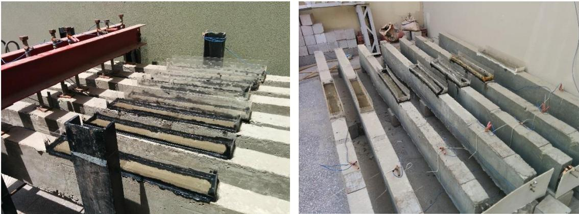
**Figure 3: Acrylic ponds fixed at the selected sections and filled with 5% NaCl**
