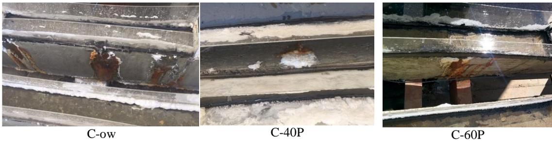
**Figure 6: Corrosion products appearing on the surface of the corroded beams**
