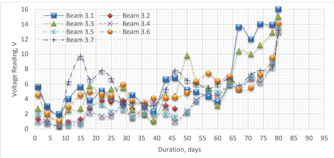
**Figure 9: Voltage readings (Volts) vs. duration (days) for the C-60P beams**
