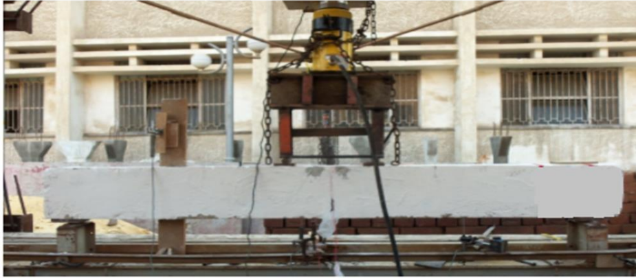
Fig. 4- Experimental Setting for Specimen Testing by Abd-Alkhalik 9
