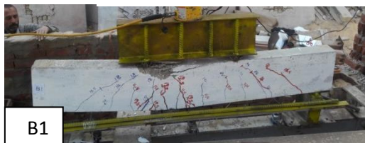
Fig. 45 Failure mode of all strengthened and non-strengthened beams
