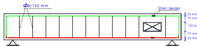
Fig. (2) Detailing of reinforcement steel for beam (B2) with opening without strengthening.
