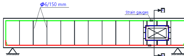
Fig. (9) Detailing of reinforcement steel for strengthening beam (B8).
