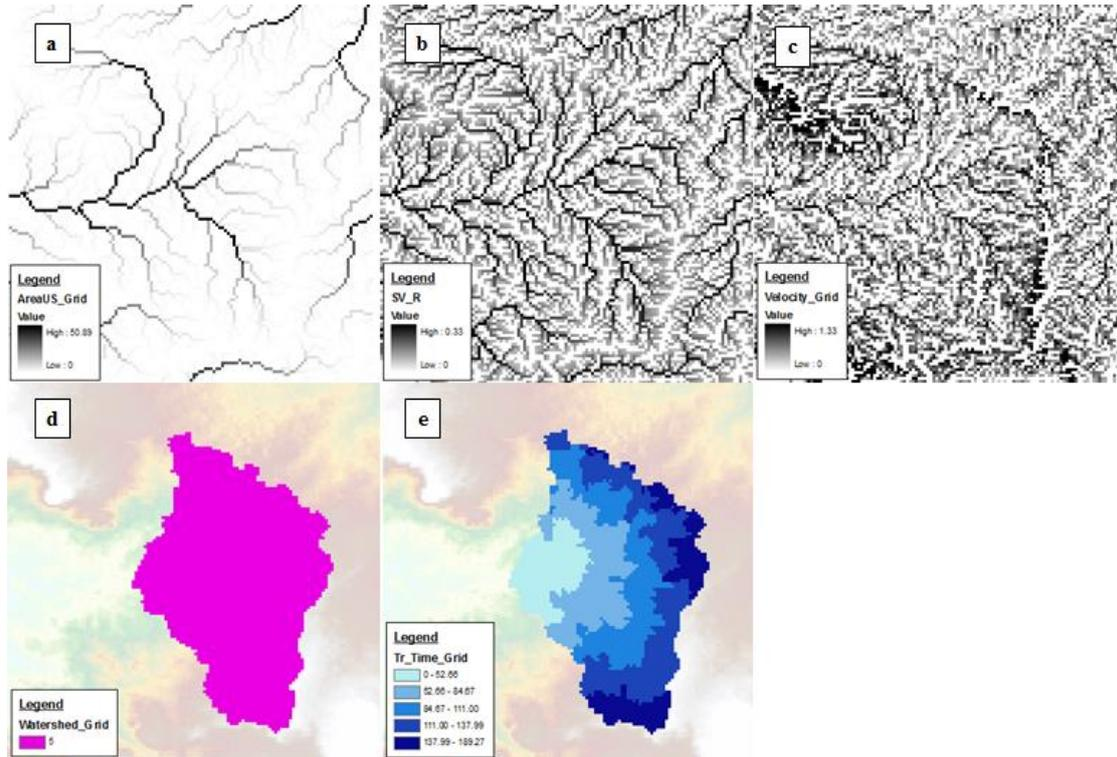
Figure (2): Example of the raster grids generated inside STA-UH model. a) Aus Grid (Km<sup>2</sup>), b) RGrid (m), c) VGrid (m/s), d) Watershed Grid and e) TGrid (min.)
