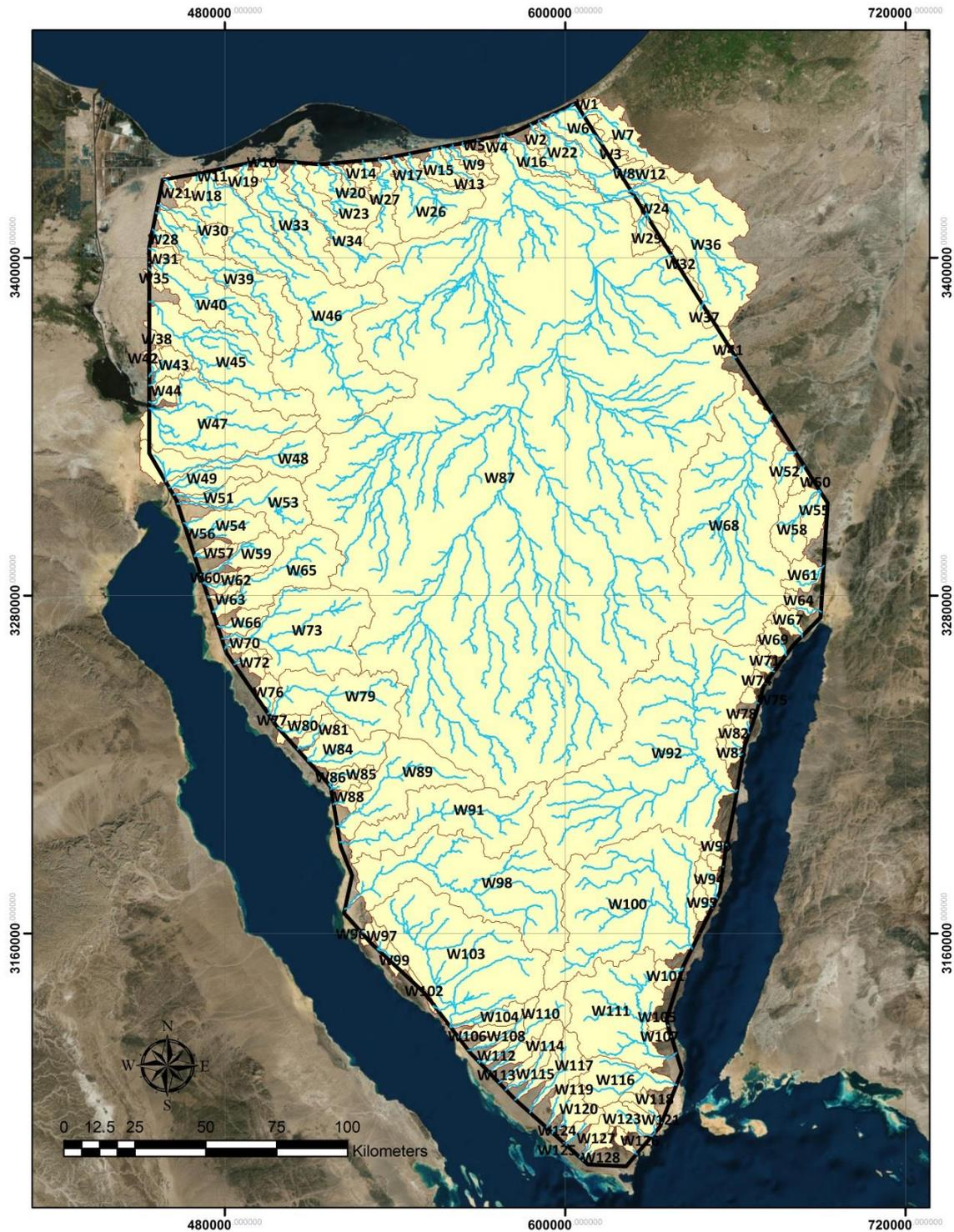
Figure (5): The 128 watersheds automatically simulated by STA-UH for Sinai Peninsula
