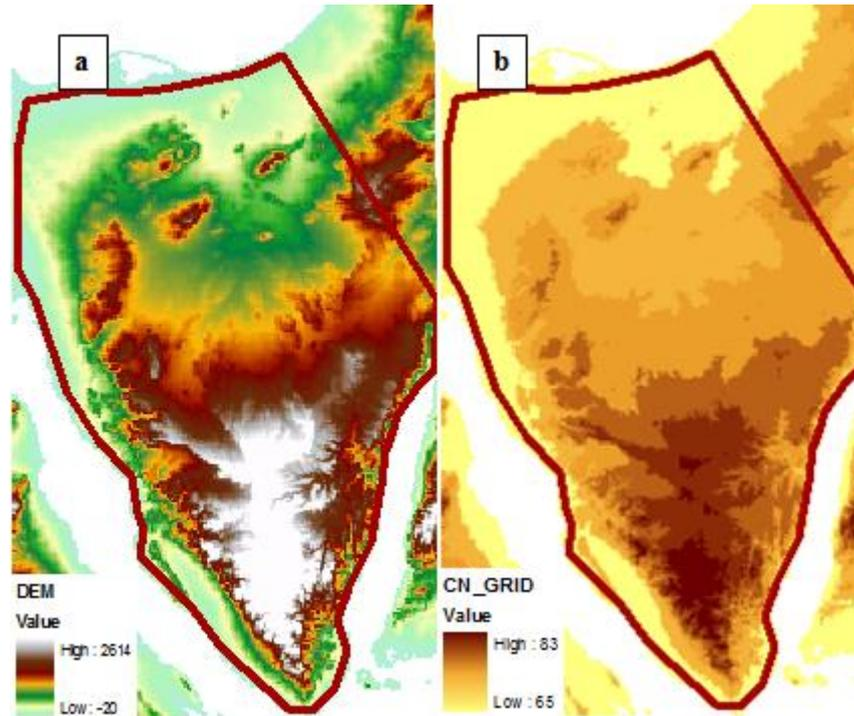
Figure (4): STA-UH input data used to simulate the whole Sinai Peninsula. a) DEM (m) and b) CN
