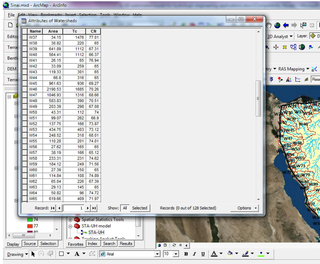
**Figure (6): The attributes table containing the hydrological parameters for each delineated watershed in Sinai Peninsula**
