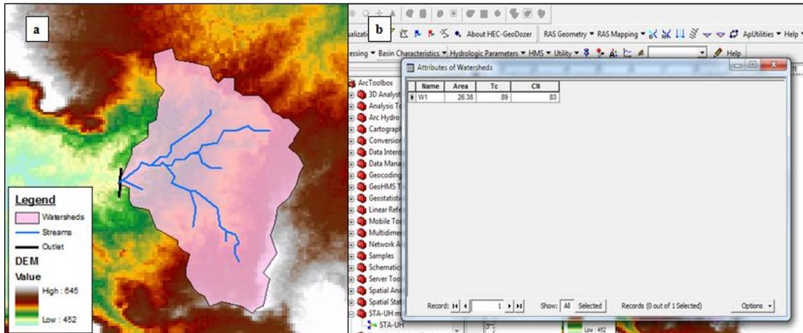
Figure (3): Sample of the STA-UH model outputs. a) Watersheds & Streams shapefile and b) Watersheds attributes table
