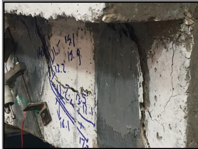
Figure 7: Crack pattern of specimen BCU-200-CAH
