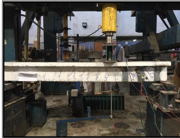
Figure 6: Crack pattern of specimen BCU-150-CAH
