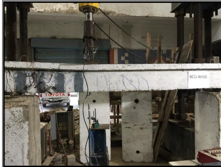
Figure 5: Crack pattern of specimen BCU-100-CAH
