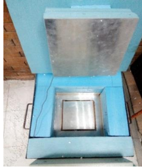
Fig. 4: Thermal conductivity test apparatus
