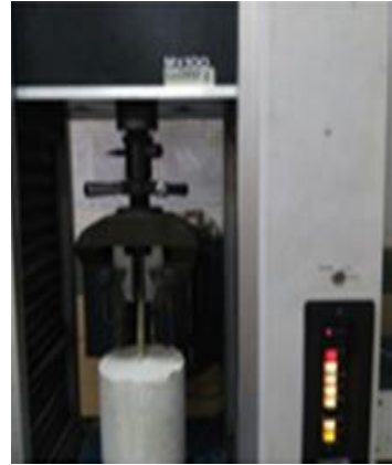
Fig. (16). Pull-out test for C.GFRP
