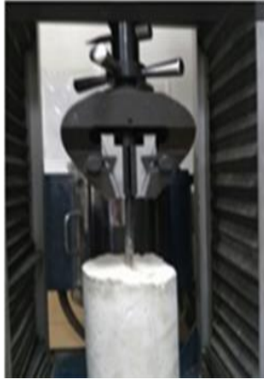
Fig. (15). Pull-out test for C.GFRP
