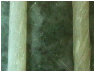
Fig. (7) 12 mm of GFRP bars
