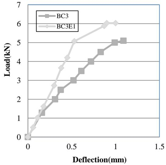
Fig. (6) Load- deflection curve of beams (BC3,BC6). Fig. (7) Load- deflection curve of beams (BC3,BC3E1).
