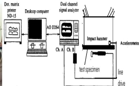
**Fig. 2 Set up for dynamic testing [20]**
