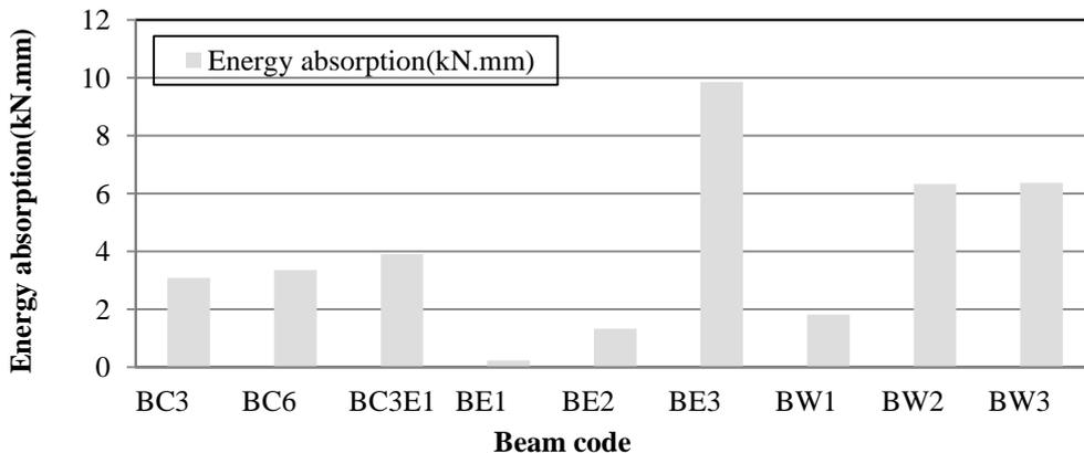
Fig. (5)The energy absorption for all test specimens
