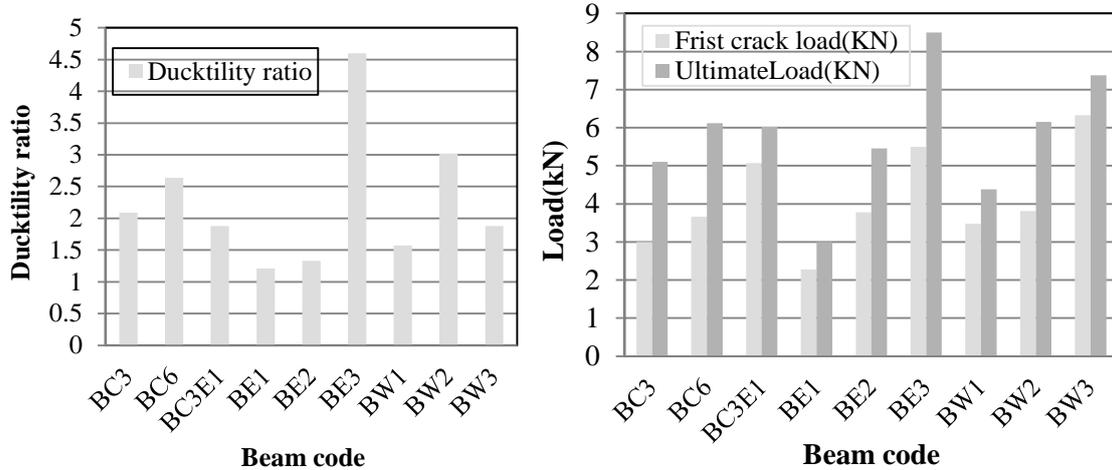
Fig. (3) The ductility ratio for beams Fig. (4)ultimate load and first crack load
