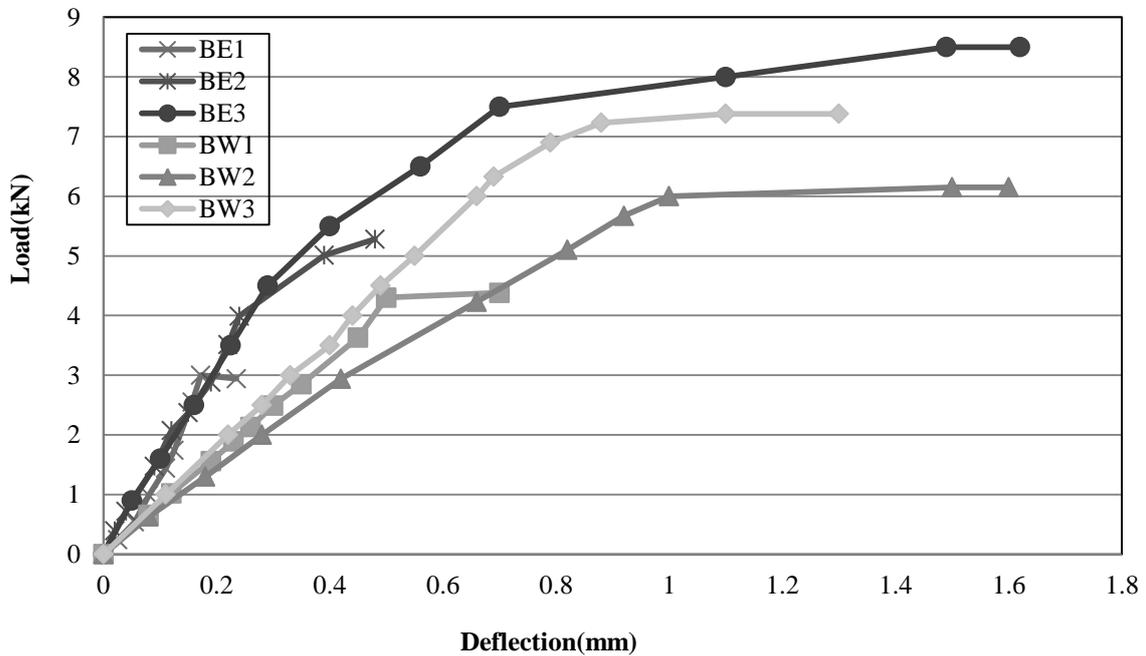
Fig. (8) Load- deflection curve of beams (BE1, BE2, BE3, BW1, BW2, BW3).
