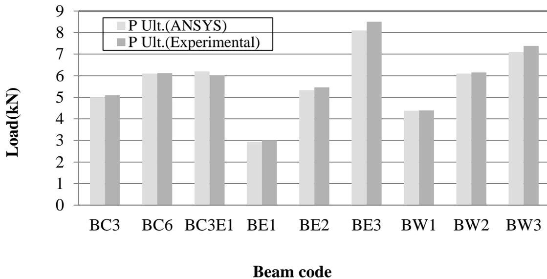
Fig(11) Difference between ultimate load bY experimental and ANSYS.
