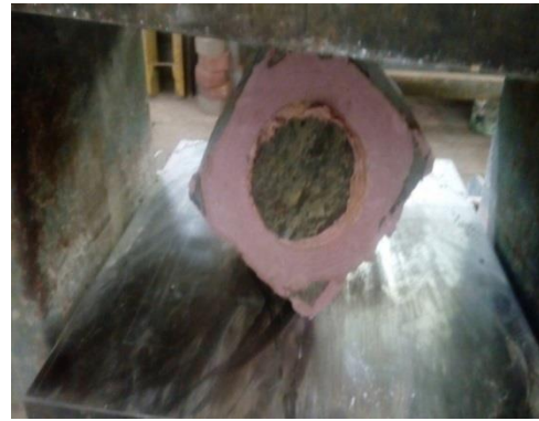
Figure (9) Specimen extracted from Permeability Equipment
