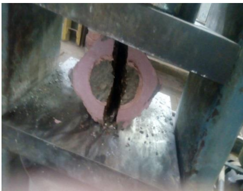
Figure (10) specimen after Splitting Test
