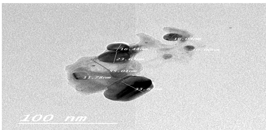
Figure (4): TEM micrograph of NK mean size particles 24nm
