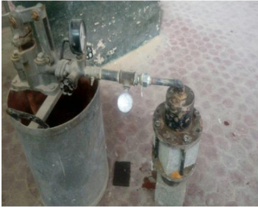
Figure (7) Water Permeability Equipment
