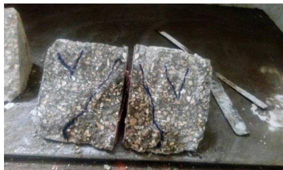
Figure (11) water penetration depth
