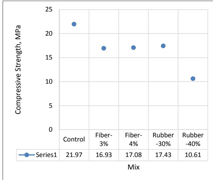
**FIGURE 9-a.** Average compressive Strength for 0% Fly Ash at 28 days
