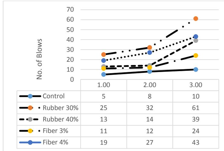
**FIGURE 10.** No. of impact blows inducing First Crack for 0% Fly Ash
