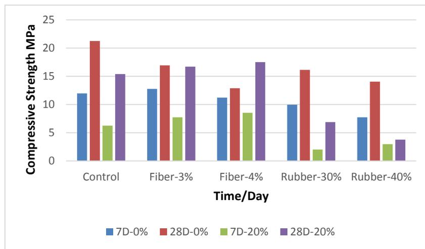
FIGURE 6. Compressive Strength comparison for 7D & 28D
