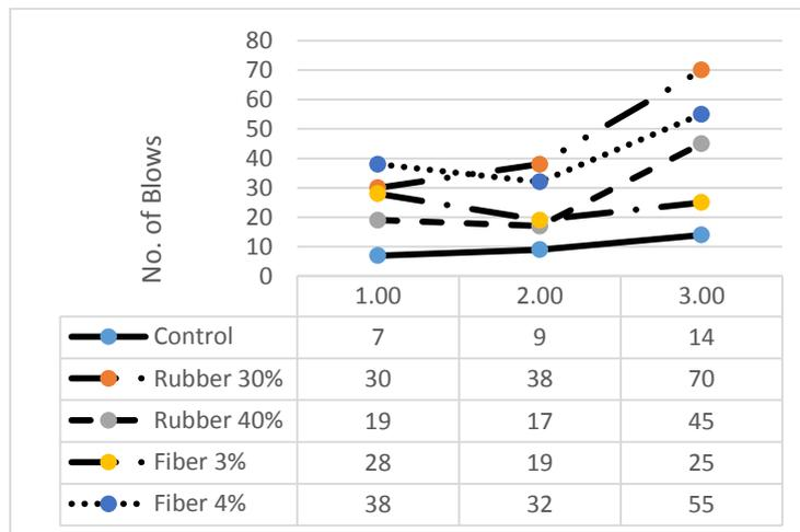
**FIGURE 11.** No. of impact blows causing failure for 0% Fly Ash
