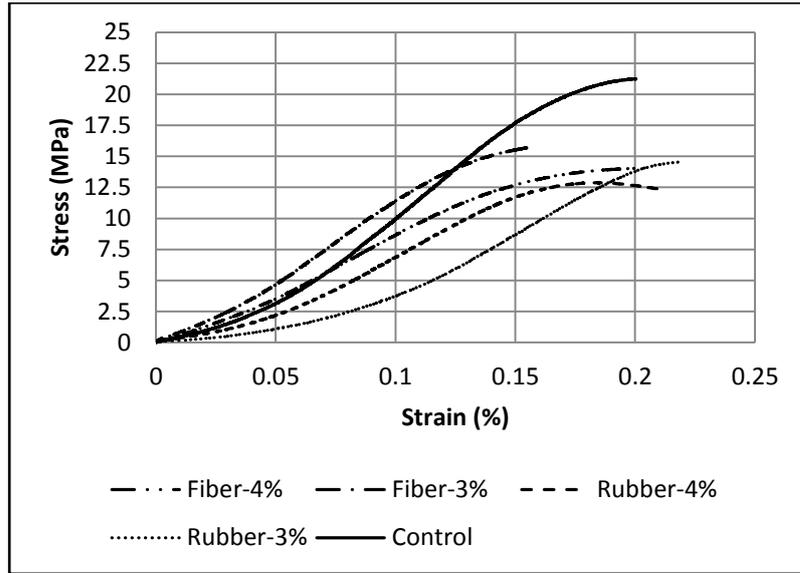
**FIGURE 7.** Stress-Strain curve at 28 days for 0% Fly Ash specimens
