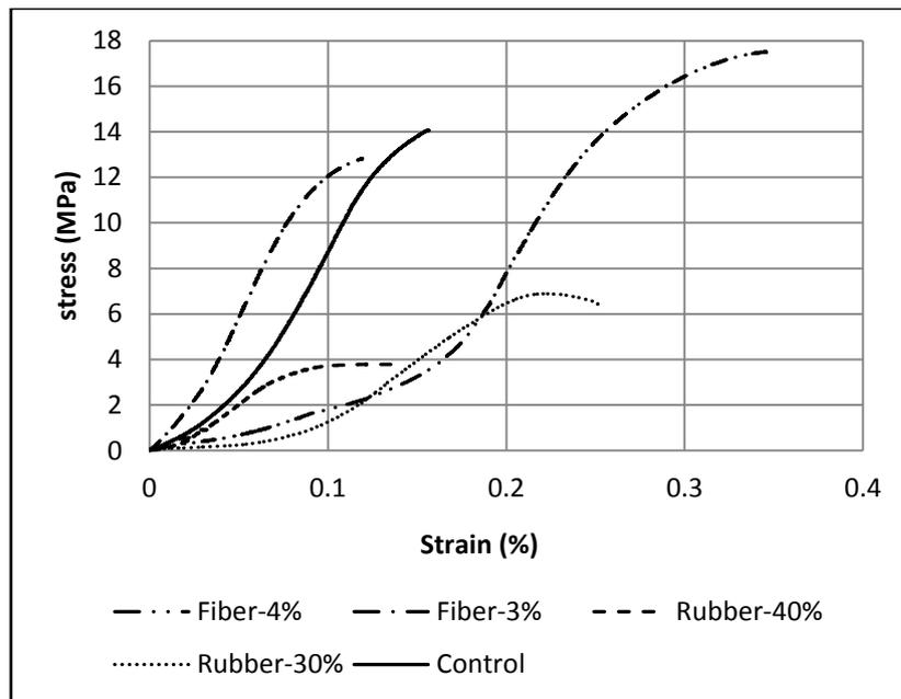
**FIGURE 8.** Stress-Strain curve at 28 days for 20% Fly Ash specimens
