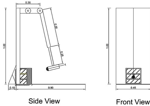
FIGURE 4. Schematic diagram for the used device, units in meter
