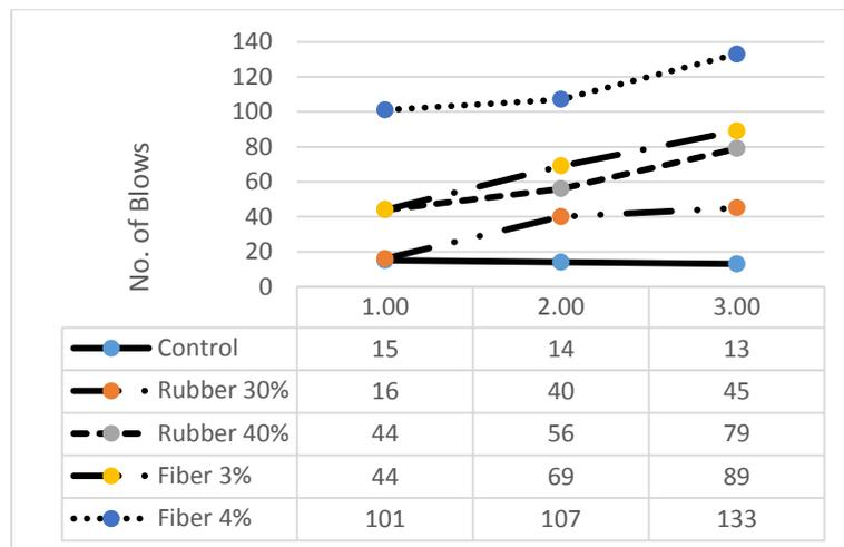
**FIGURE 13.** No. of impact blows causing failure for 20% Fly Ash
