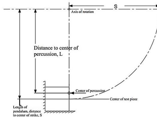
FIGURE 3. Free body diagram for the conducted test
