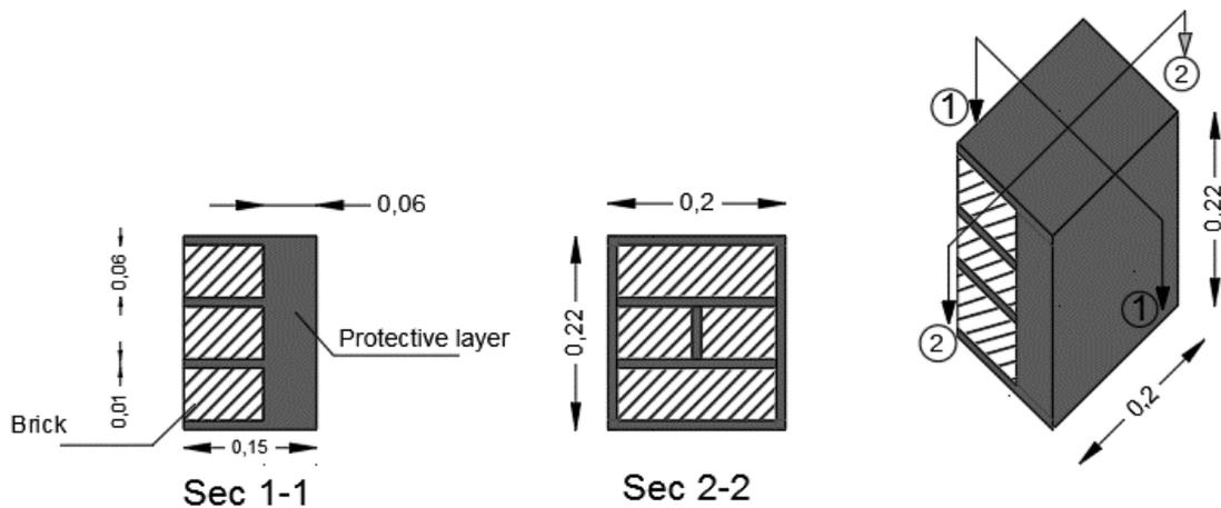
FIGURE 5. Tested Sample schematic diagram, units in meter
