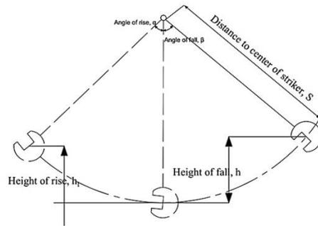
FIGURE 2. Charpy test free body diagram
