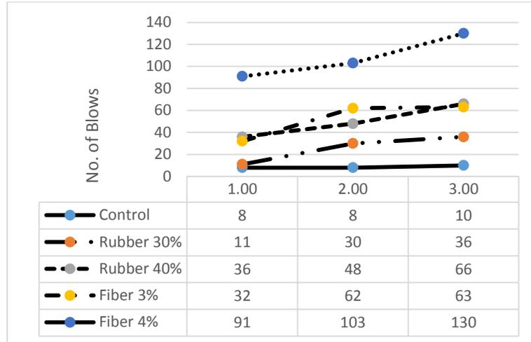
**FIGURE 12.** No. of impact blows inducing First Crack for 20% Fly Ash
