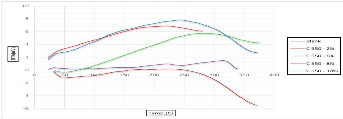
Fig. (7): DTA-Temp. Curve of Reference and C550 specimens at 400°C.
