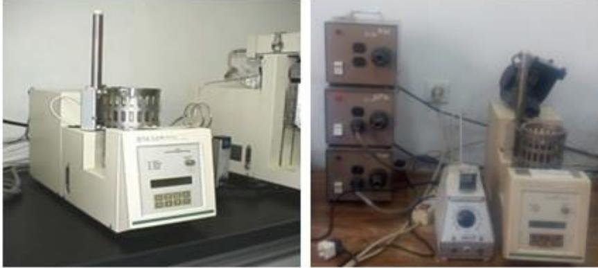
Figure(3): Differential Thermal Analyzer (DTA) to determine thermal properties and melting point for samples
