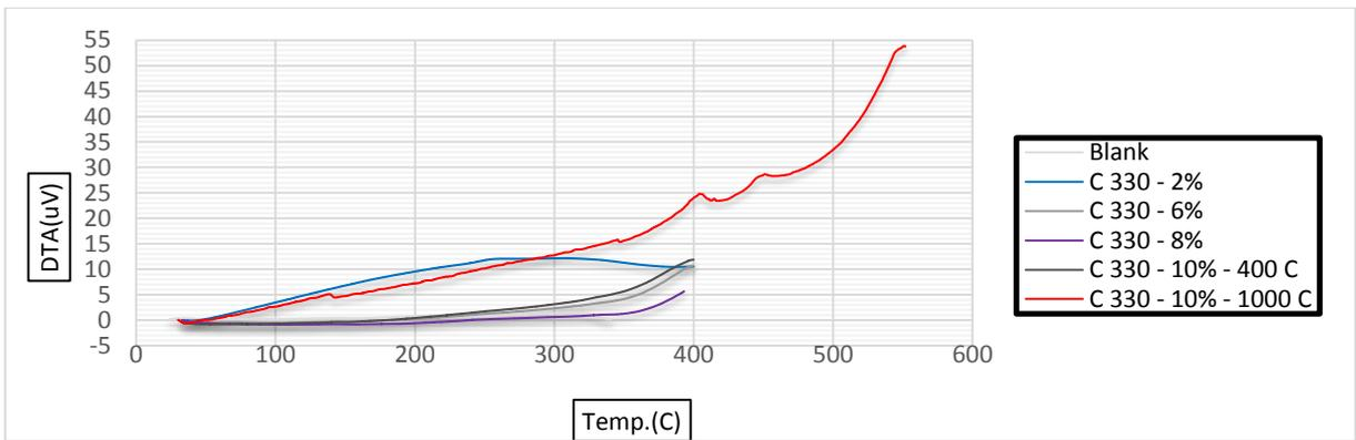
Fig. (5): DTA-Temp. Curve of C330 specimens at 1000°C.
