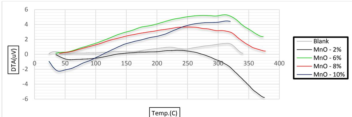
Fig. (12): DTA-Temp. Curve of Reference and MnO specimens at 400°C.
