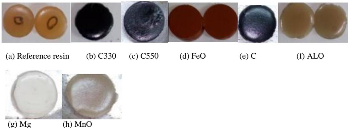
Fig. (2): Tested specimens of resin with 10 mm diameter and 5 mm height by DTA at Micro Analytical Center of Cairo University.
