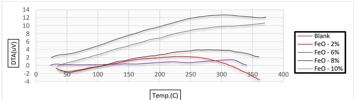
Fig. (8): DTA-Temp. Curve of Reference and FeO specimens at 400°C.
