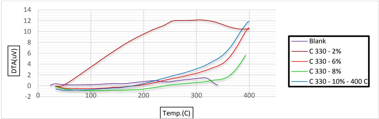
Fig. (4): DTA-Temp. Curve of Base resin and C330 specimens at 400°C.
