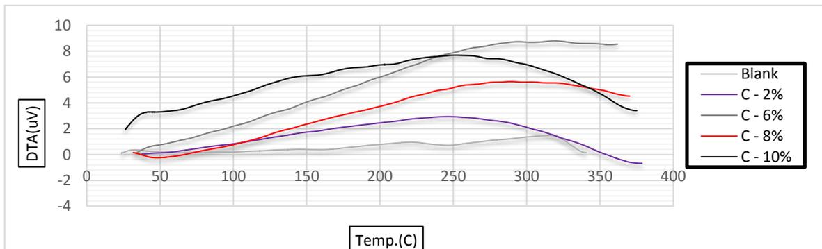
Fig. (9): DTA-Temp. Curve of Reference and C specimens at 400°C.
