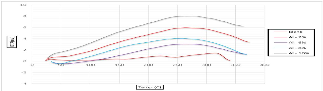
Fig. (10): DTA-Temp. Curve of Reference and ALO specimens at 400°C.
