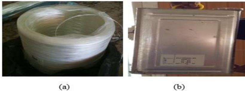
Fig. (1): (a) Glass fiber roving – (b) package of polyester
