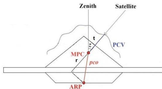
Fig. (1): Diagram of locations of the GNSS antenna phase center variations modified from Dawidowicz (2010).
