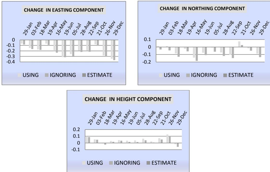
Fig. (24): Changing in the three coordinates components (Easting, Northing and Height) in one day of each month for station ALAM.
