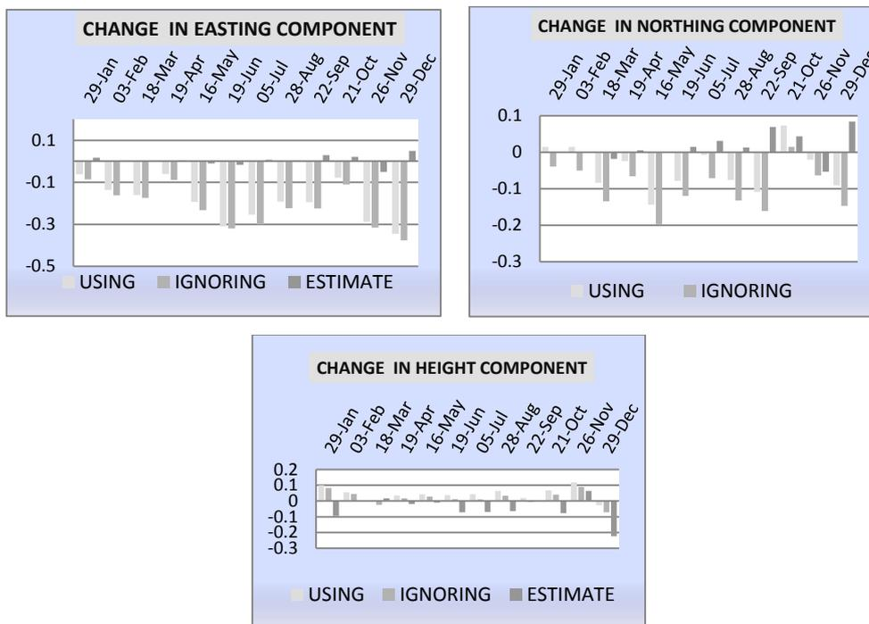
Fig. ( 25 ): Changing in the three coordinates components (Easting, Northing and Height) in one day of each month for station ASWN.
