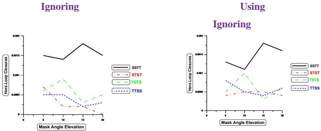
Fig. (12): Minimum length of loop for horizontal loop closure error.
