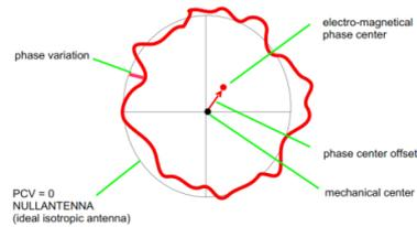
Fig. (2): Variations and offset of antenna phase center (PCV) modified from Schmitzey al, (2017).
