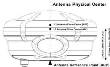
Fig. (3): Location of two phase center for L1, L2 frequencies modified from El-Hattab (2013).
