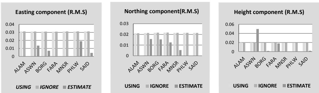
Fig. (27): R.M.S in Easting, Northing and Height components due to antenna phase center for day Dec 30.
