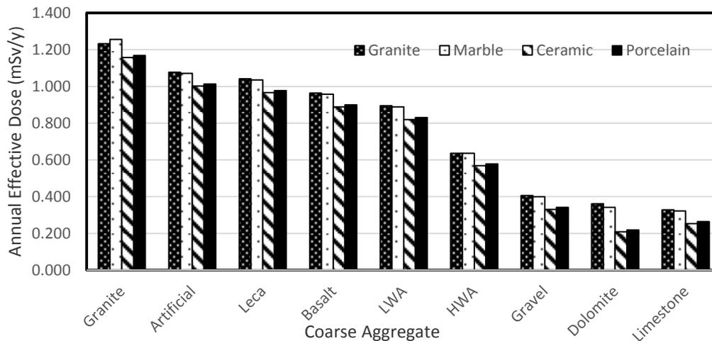
FIG.20 Effect of Aggregate and Floor Finishing on Annual Effective Dose (Clay Bricks)
