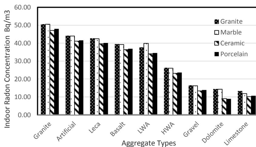
**Fig. 14 Effect of Aggregate and Floor Finishing on Indoor Radon Concentration (cement bricks)**
