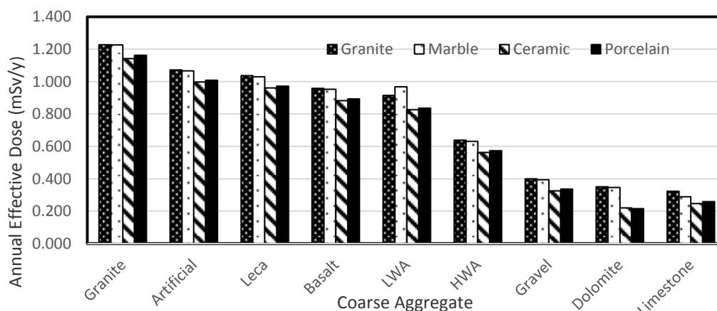
FIG. 19 Effect of Aggregate and Floor Finishing on Annual Effective Dose (Cement Bricks)
