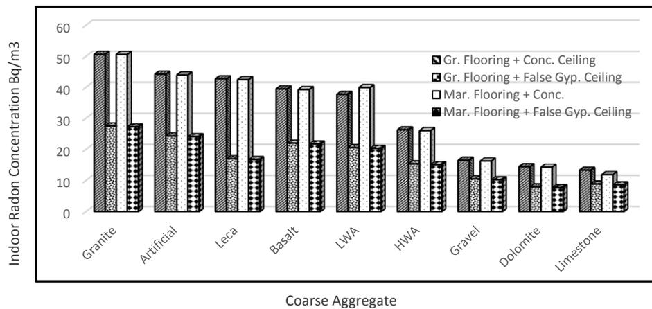
**FIG. 16 The Effect of Gypsum False Ceiling on Indoor Radon Concentration**
