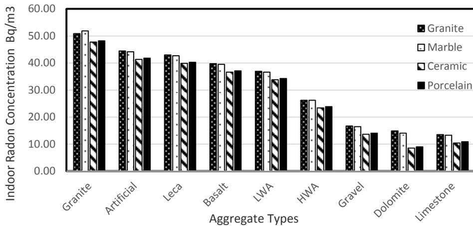
**Fig. 15 Effect of Aggregate and Floor Finishing on Indoor Radon Concentration (clay bricks)**
