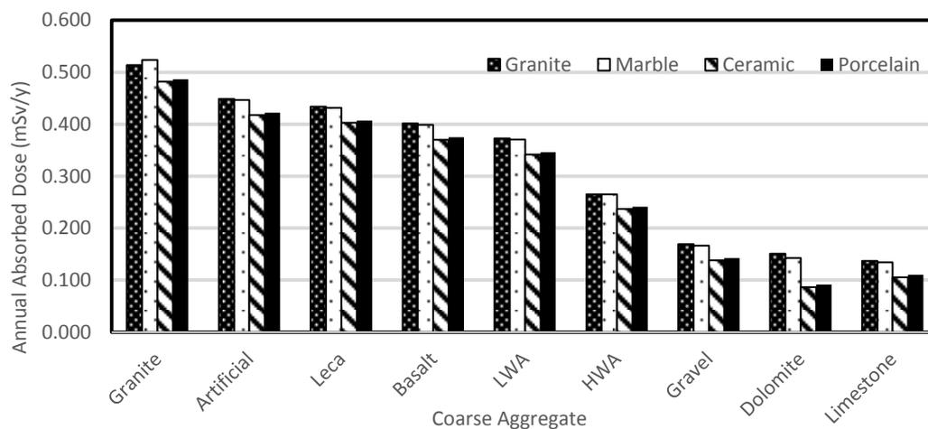
FIG. 18 Effect of Aggregate and Floor Finishing on Annual Absorbed Dose (Clay Bricks)
