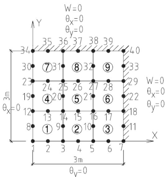
**Fig. ( 4 )** A Quarter of Clamped Square Plate Discretized into mesh 3x3 using Heterosis element
