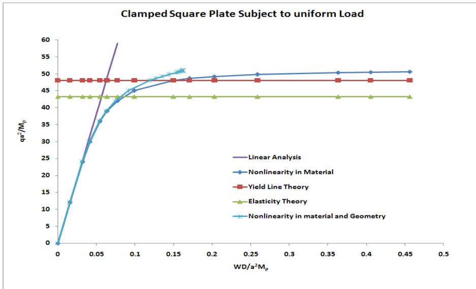
Fig. (8) Load-Deflection Curve for Clamped Square Plate Subjected to Uniform Load
