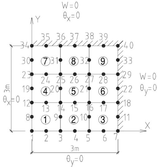
**Fig. ( 5 ) A Quarter of Simply Supported Square Plate Discretized into mesh 3x3 using Heterosis element**
