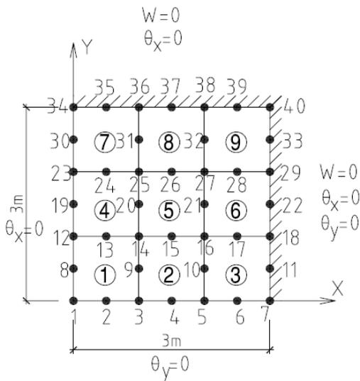
**Fig. ( 6 ) A Quarter of Two Opposite Edges Clamped and Other One Simply Supported Square Plate Discretized into mesh 3x3 using Heterosis element**
