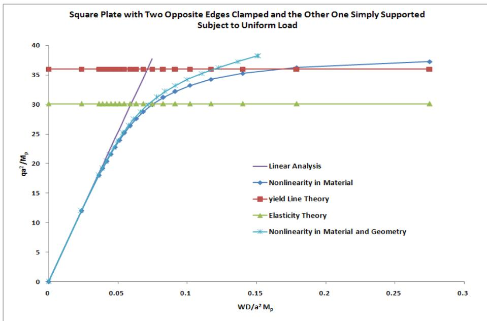
Fig.(9) Load-Deflection Curve for Square Plate with Two Opposite Edges Clamped and Other Ones Simply Supported Subjected to Uniform Load
