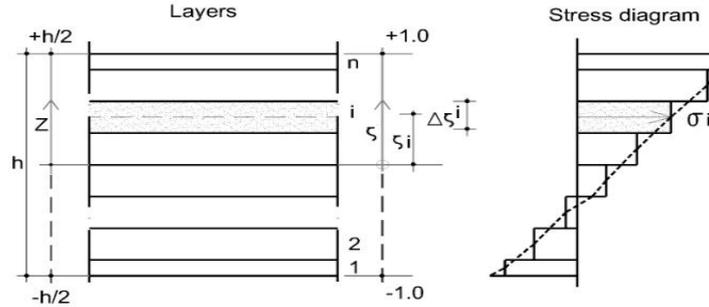
**Fig.( 3) Layered Subdivision of Plate and the Corresponding Stress**
