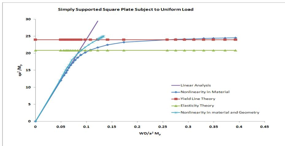
**Fig. (7) Load-Deflection Curve for Simply Supported Square Plate Subjected to Uniform Load**
