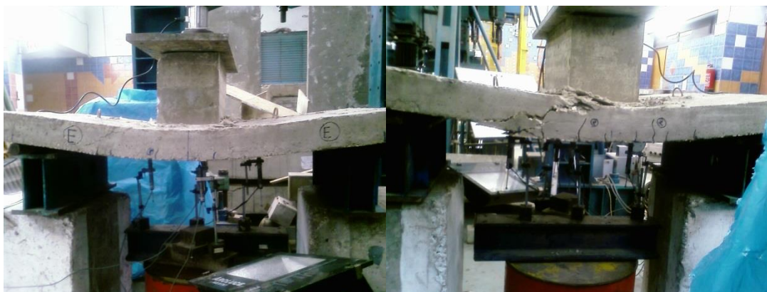
Fig. (14): Flexure failure occurs accompanied with shear failure at final stage
