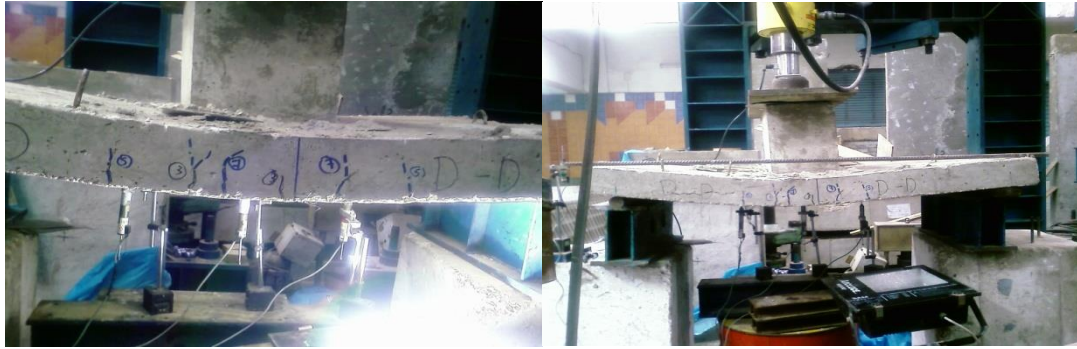
Fig. (12): Flexure failure occurs accompanied with minor shear cracks at final stage.
