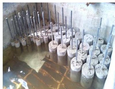
**Figure 2. Lollipop Samples after Casting and Curing Process**
