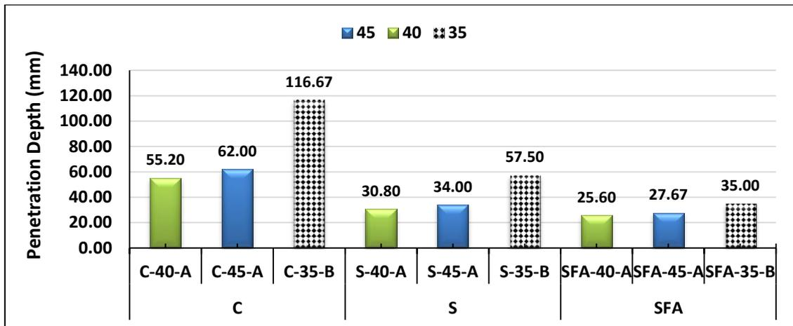
Figure 15. Average Water Depth after Permeability Test
