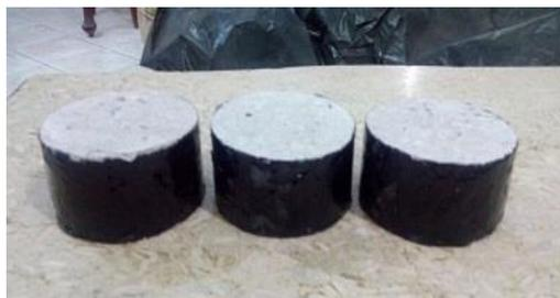
**Figure 5. Concrete Specimens Coated and Prepared**
