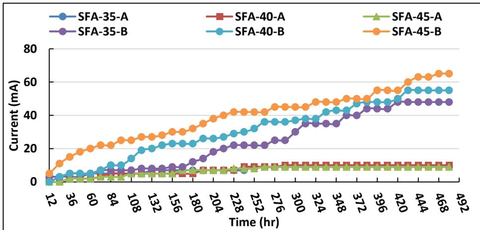
Figure (12.c) Current (mA) for (CEM III/A + 20% FA) Mixtures (10cm diam.)
