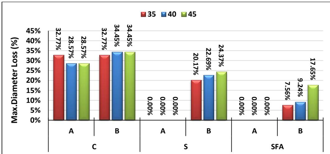
Figure (17.b) Percentage of Max. Diameter Loss for Lollipop Specimens (10cm Diam.)
