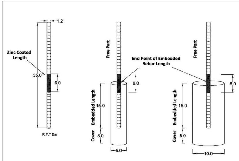
**Figure 1. Schematic Diagram of Lollipop Specimens Design (Dimensions are in cm)**
