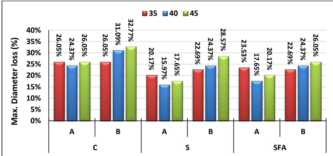
Figure (17.a) Percentage of Max. Diameter Loss for Lollipop Specimens (5cm Diam.)
