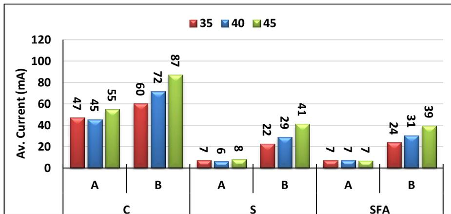
**Figure 14.b) Average of Measured Current (mA) for Lollipop Specimens with (10cm diam.)**
