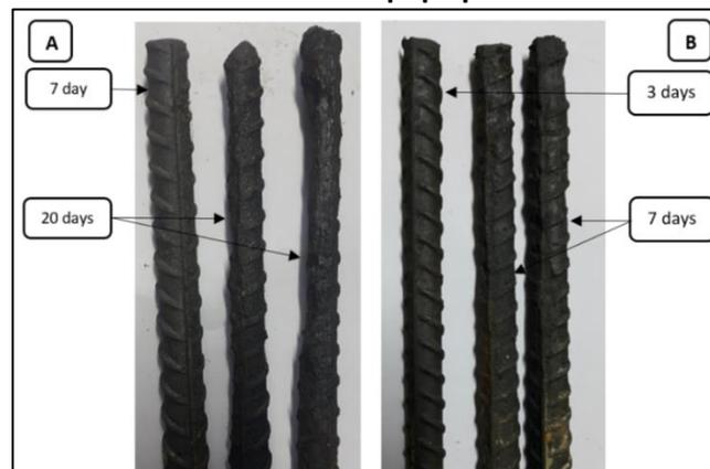
**A:** Rebars Extracted from 10cm diameter specimens cast with (CEM I)
