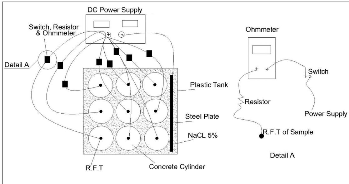
**Figure 3. Schematic Diagram of Impressed Current Test Method for Lollipop Samples**
