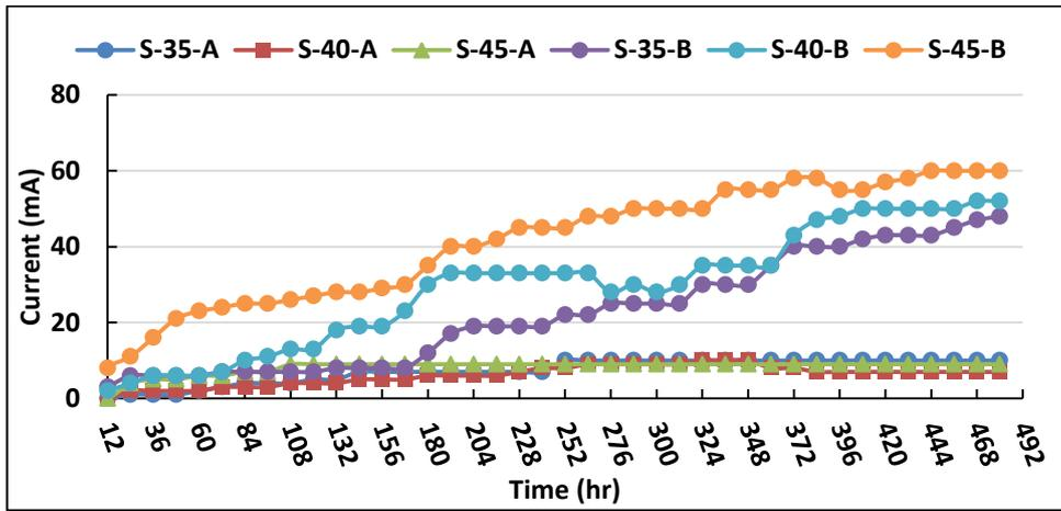
Figure (12.b) Current (mA) for CEM (III/A) Mixtures (10cm diam.)
