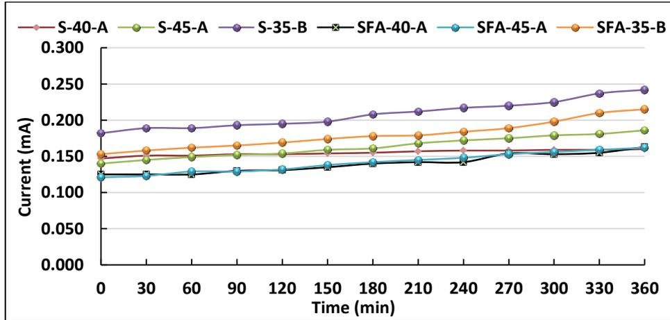
Figure (16.b) Current Passed Through Specimens during All 6-Hours For (CEM III/A, and CEM III/A + 20% FA) only
