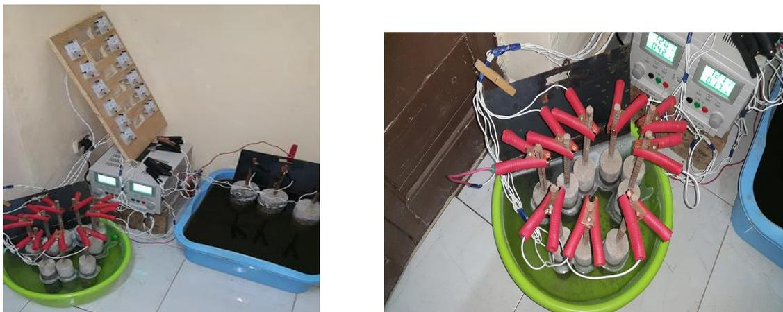
**Figure 4. Test Setup Contains (DC Power Supply, 2 Plastic Containers, and Ohmmeter Board)**
