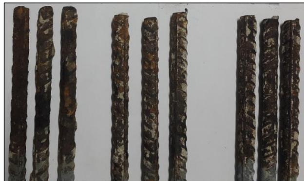
**Figure 7. Extracted Rebars from Lollipop Specimens before Cleaning**
