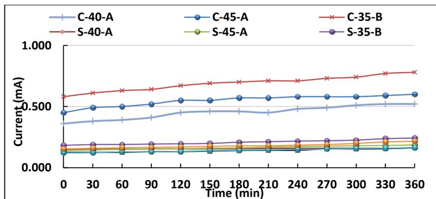
Figure (16.a) Current Passed Through All the Specimens during All 6-Hours
