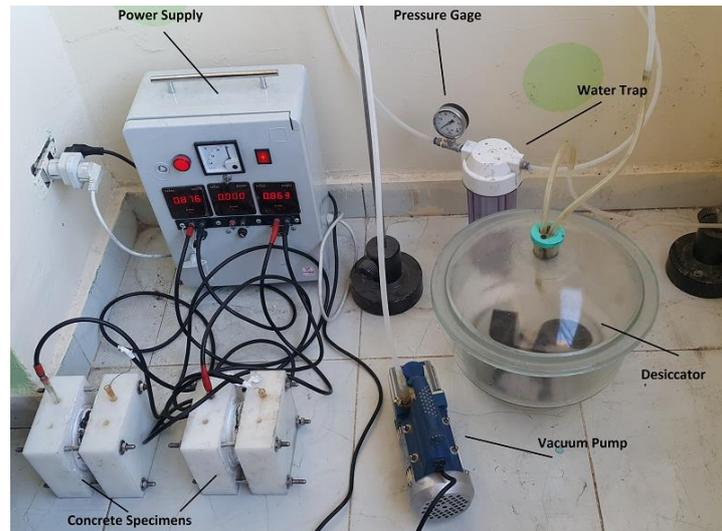
**Figure 6. Rapid Chloride Penetration Test and Preparation Phases**
