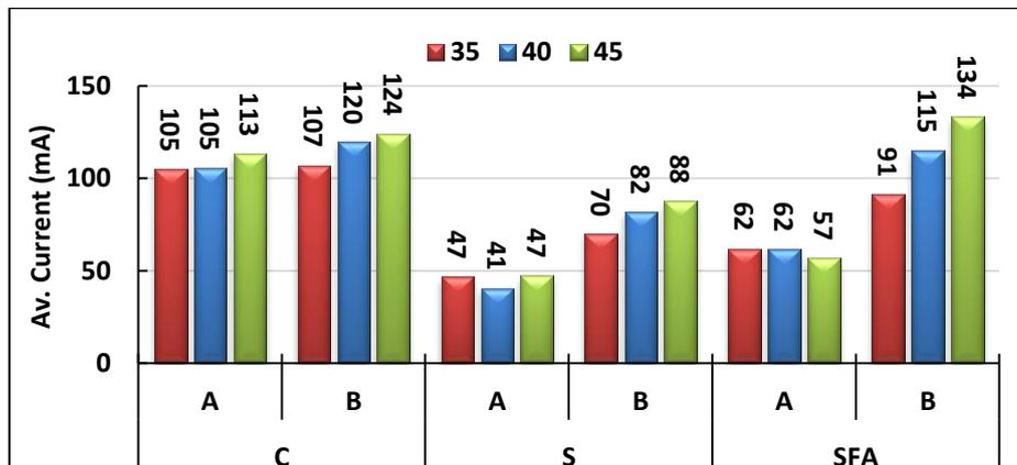
**Figure 14.a) Average of Measured Current (mA) for Lollipop Specimens with (5cm diam.)**
