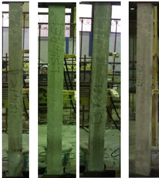
Fig. 3: Column specimens after curing.
