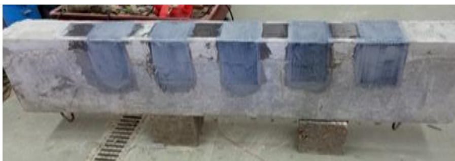
Fig. 2: Strengthening configuration of B6
