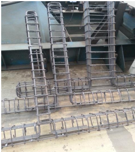
Figure 1-a: Steel Reinforcement of specimens
