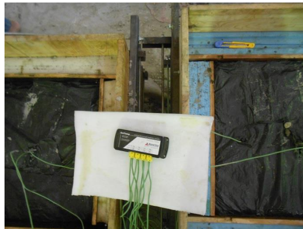
Figure 3: Connecting Thermocouples Wires to Data Logger
