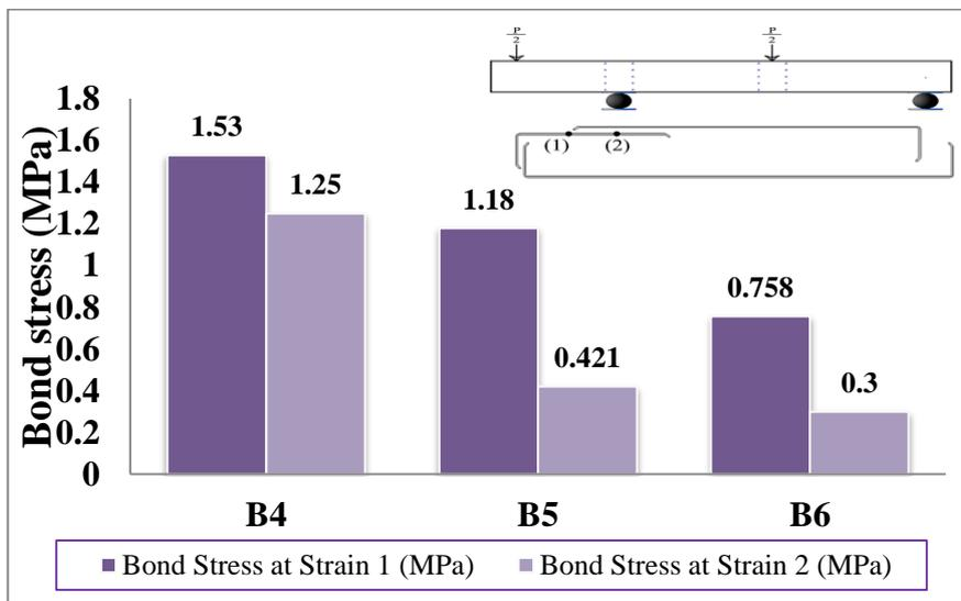
**Fig 15** Bond Stress Along Lap Splice at Strain 1 and 2 for Group 2 (B4,B5,B6)
