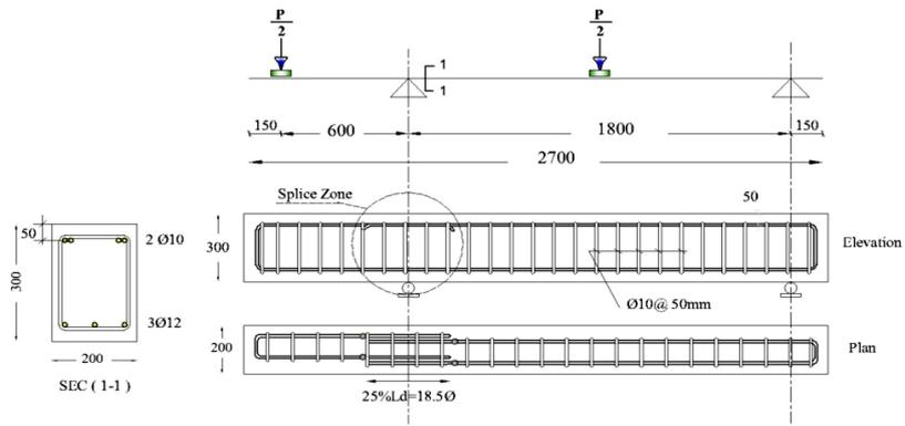
**Fig.6** Geometry and dimensions of Group 4
