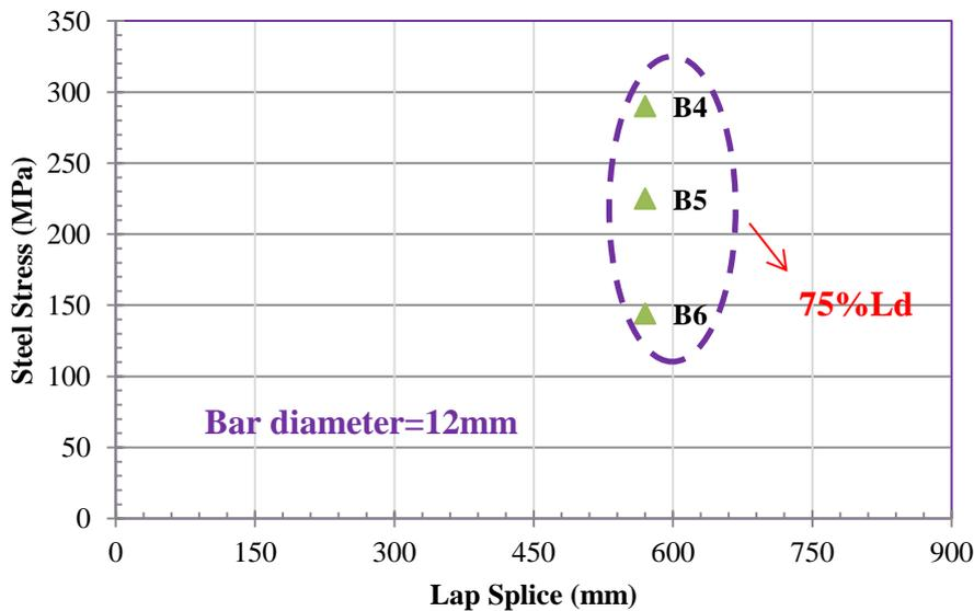
**Fig 13** The Relation Between The Steel Stress and The Splice Length of Group 2
