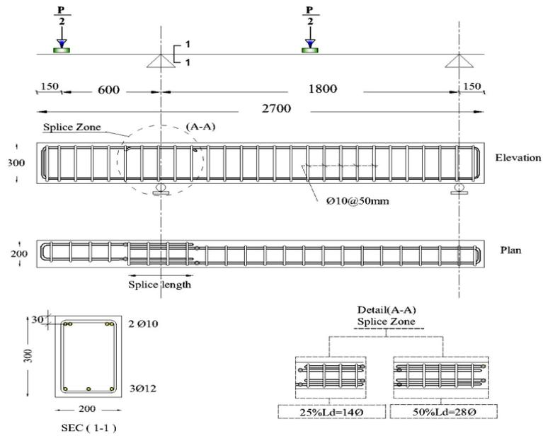
**Fig.6** Geometry and dimensions of Group 5
