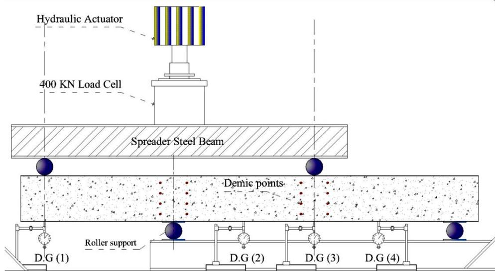
**Fig.2** Test setup
