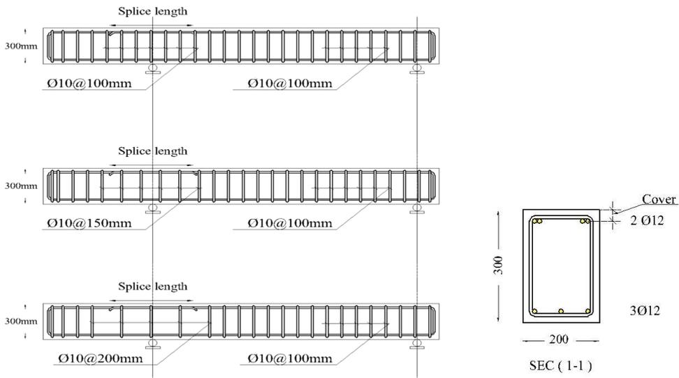
**Fig.4** Geometry and dimensions of Group 2
