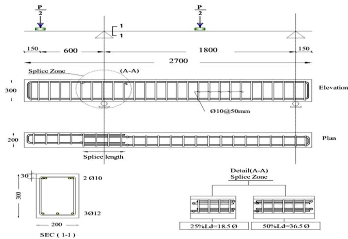
**Fig.7** Geometry and dimensions of Group 6
