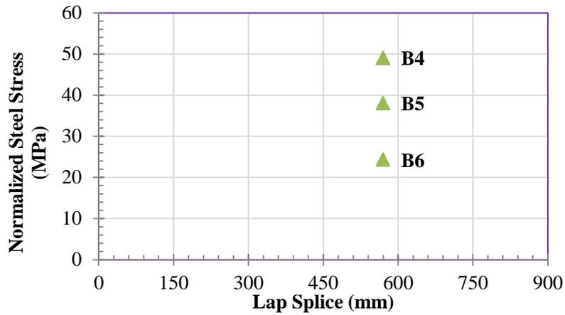
**Fig 14** The Relation Between The Normalized Steel Stress and The Splice Length of Groups 2
