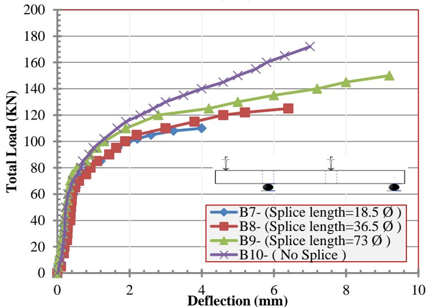
**Fig 9** Beams (B7,B8 ,B9 ,B10): Load-Deflection curve at D.G1
