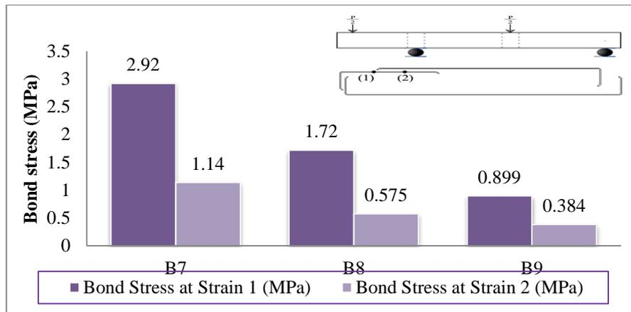
**Fig 11** Bond Stress Along Lap Splice at Strain 1 and 2 for Group 3
