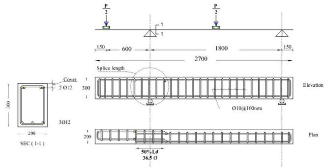
**Fig.3** Geometry and dimensions of Group 1 ( B1,B2,B3)
