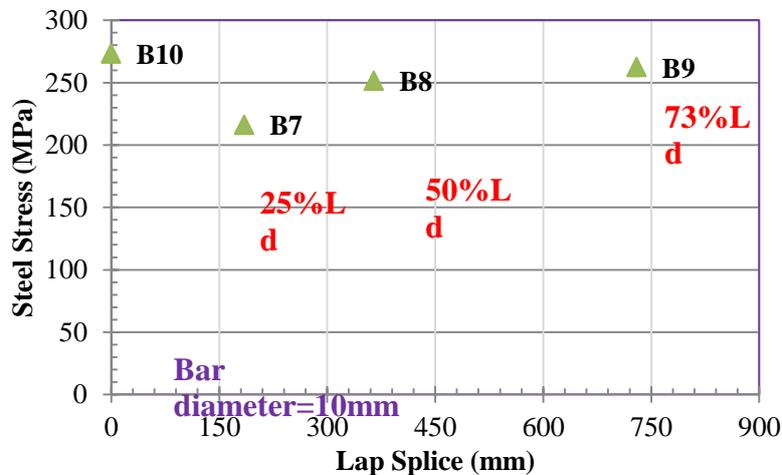
**Fig 10** The Relation Between The Steel Stress and The Splice Length of Groups 3
