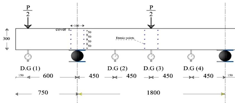
**Fig.1**The positioning of Dial gages and Demarcation points on specimens
