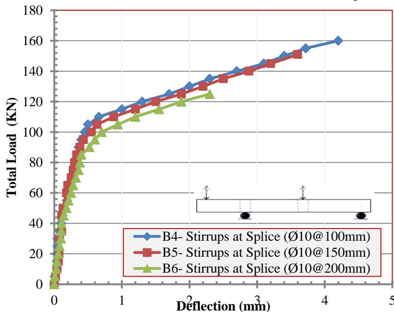
**Fig 12** Beams (B4,B5,B6): Load – Deflection curve at D.G1
