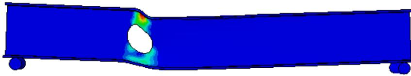
Figure 5: The deformed finite element model at failure.
