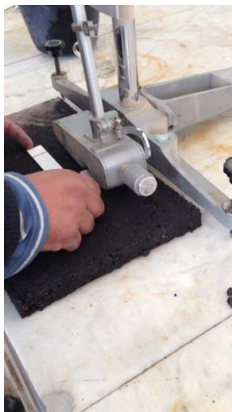
Figure (2): Portable Skid Resistance Tester contact-area specimen adjustment
