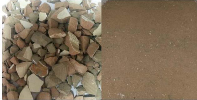
Coarse ceramic aggregate Fine ceramic aggregate Figure (1): Recycled ceramic tile waste aggregates
